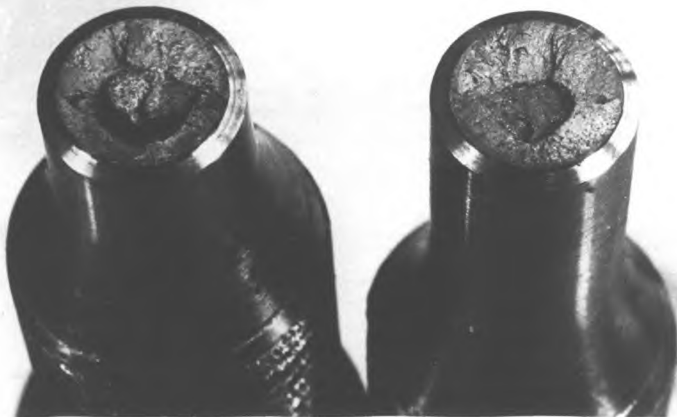
PLATE II. CRACK PROPAGATION IN CAST Cr-Mn STEEL. CB 7.
