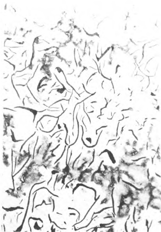
PLATE 17 MEDIUM FLAKE CAST IRON E (X 60)
