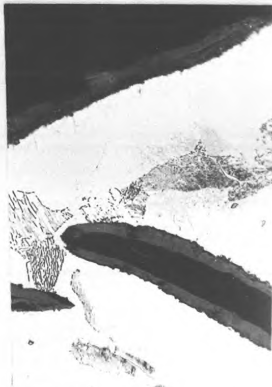
PLATE 15. COARSE FLAKE CAST IRON B (x600)
