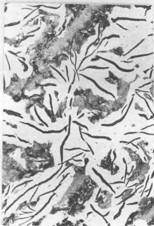
PLATE 14. COARSE FLAKE CAST IRON B' (x60)
