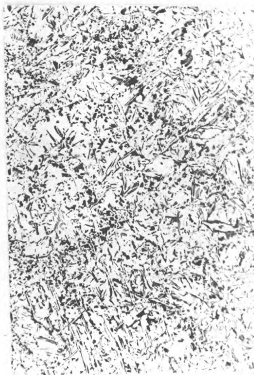
PLATE 19. CAST MILD STEEL S (X 60)
