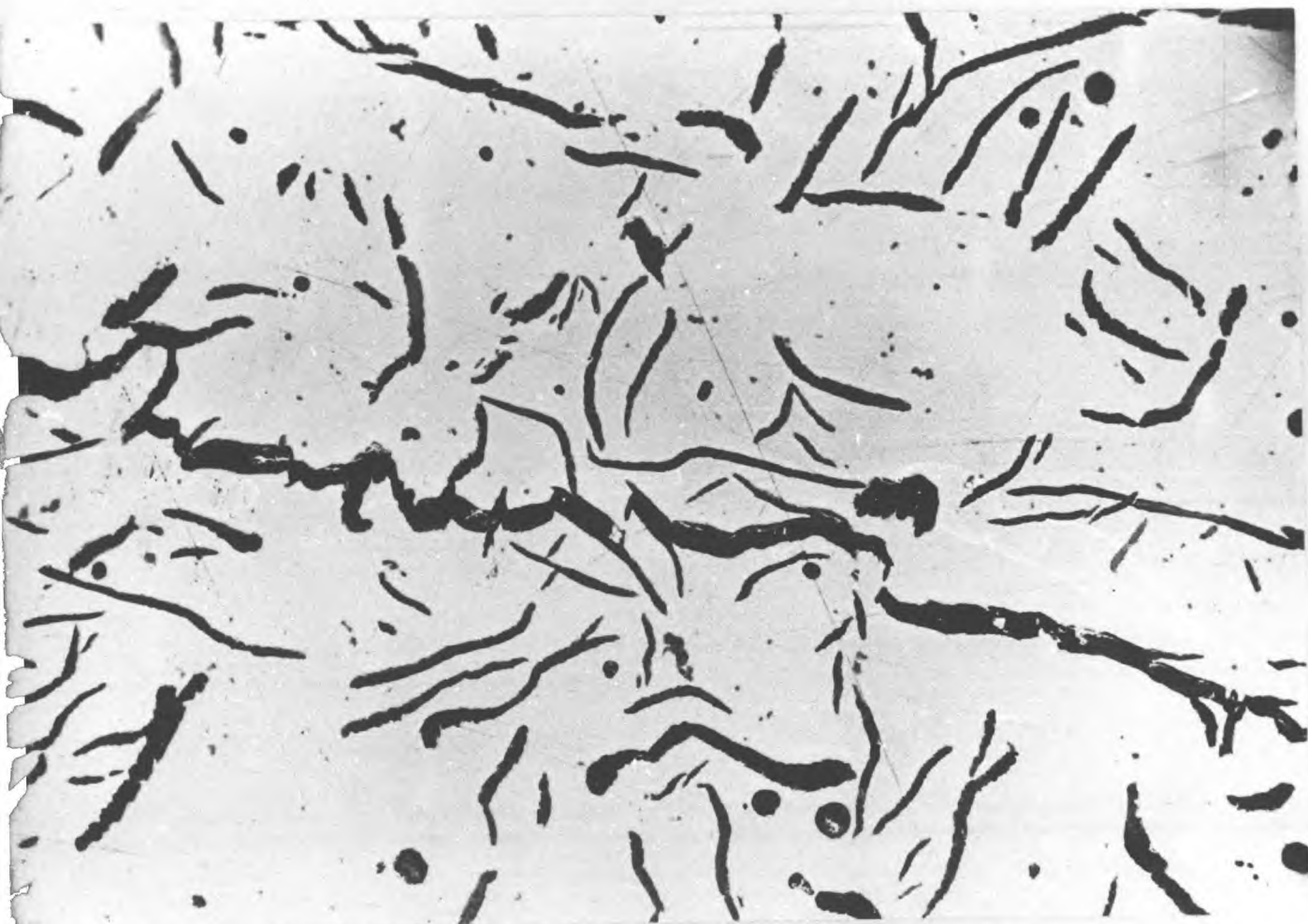
PLATE 9. FRACTURE OF FLAKE CAST IRON 7EB.8. (XGO.)
