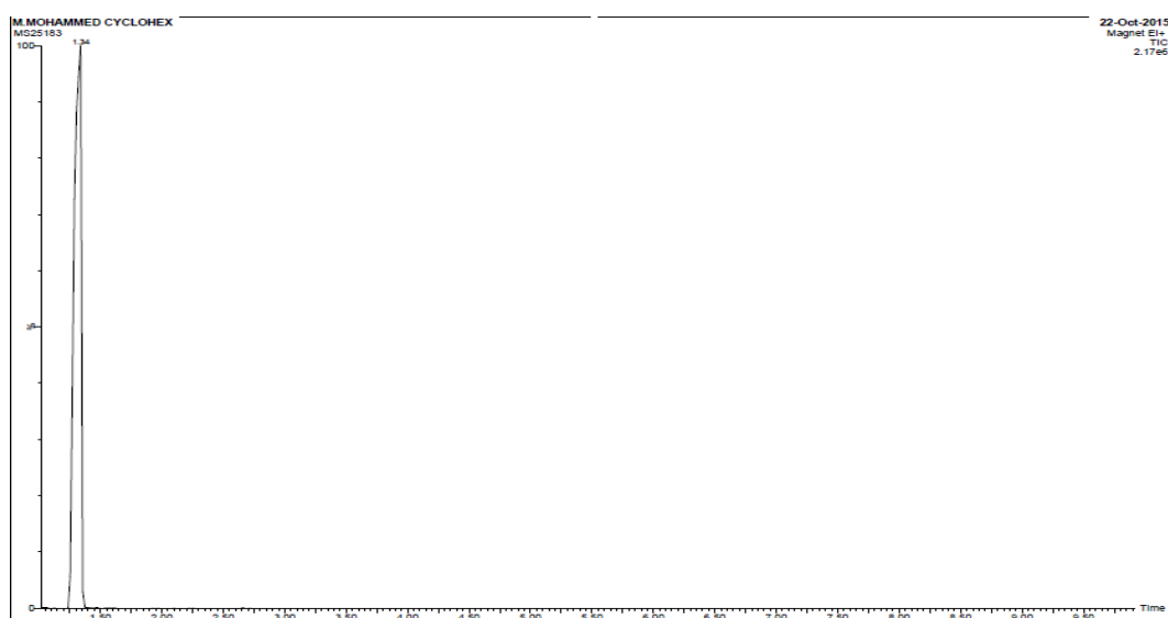
Figure 7.22: The chromatogram of the pure cyclohexane sample
