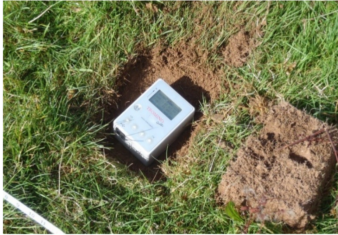
Figure 4-5: Tromino Instrument installed in a testing hole with removed earth visible on the right. On the left side of instrument an arrow can be seen which must be pointing north disregarding the direction of transect.
