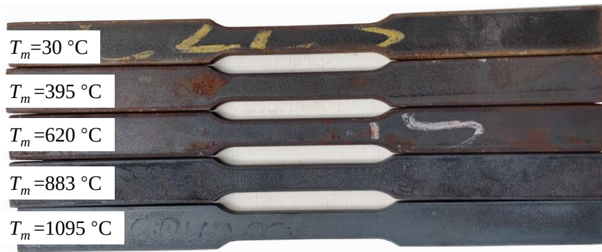
Fig. 3. Post-fire surface colors of S700 high strength steel.
