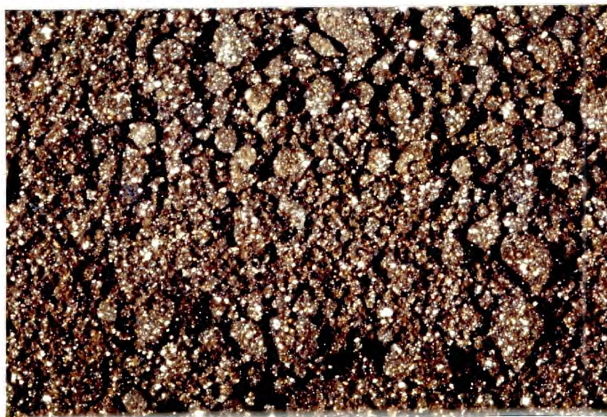
Photograph No.3: Crystalline Stannic Sulphide, \text{SnS}_2 , obtained at 600^\circ\text{C} . in sulphidizer with reducer at 700^\circ\text{C} . using high gas flow-rate and four hours reaction period (Magnification = 4\times ).
