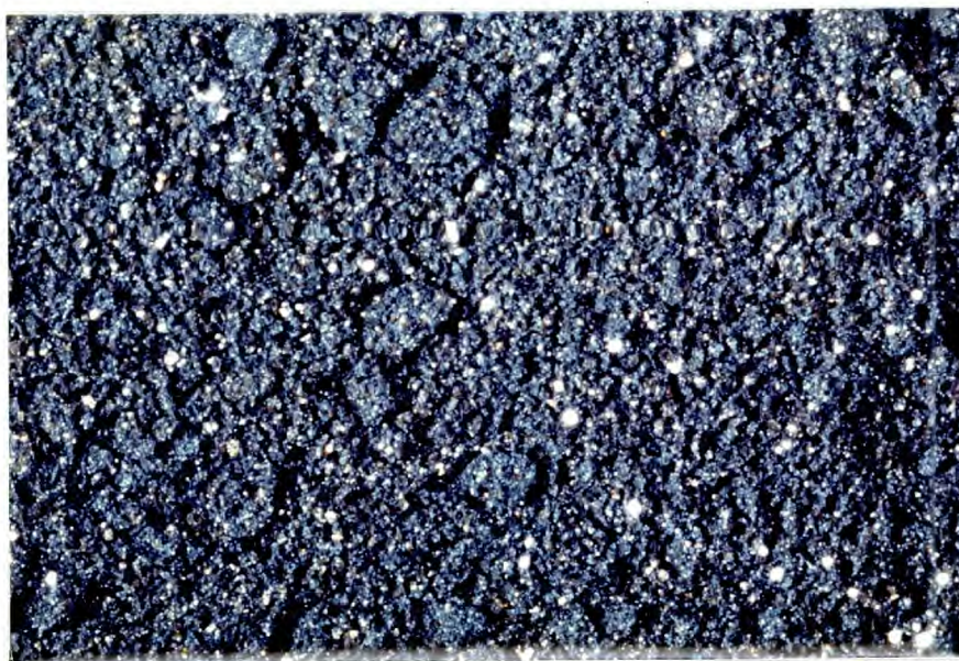
Photograph No.4: Tin Sesquisulphide, \text{Sn}_2\text{S}_3 , obtained at 620^\circ\text{C} . (Magnification = 4\times ).
