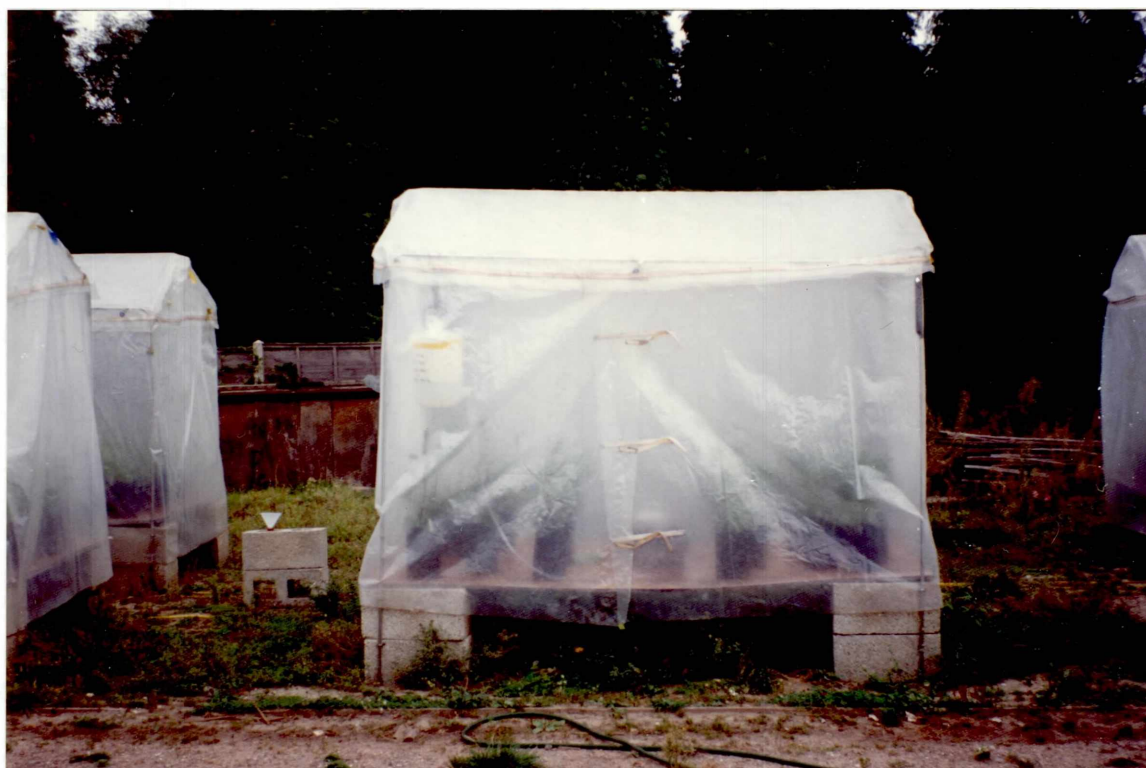
Plate 1. Temporary misting chambers for the exposure of tree seedlings.
