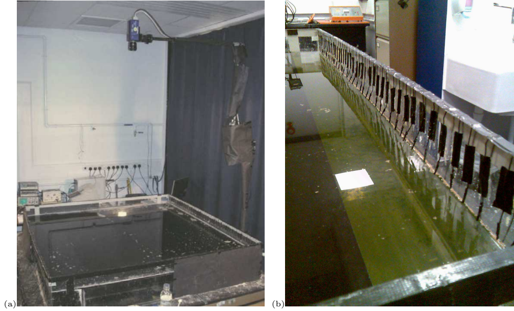
Figure 3.2: (a) Experimental rig setup and (b) electrodes at the side of the tank.
