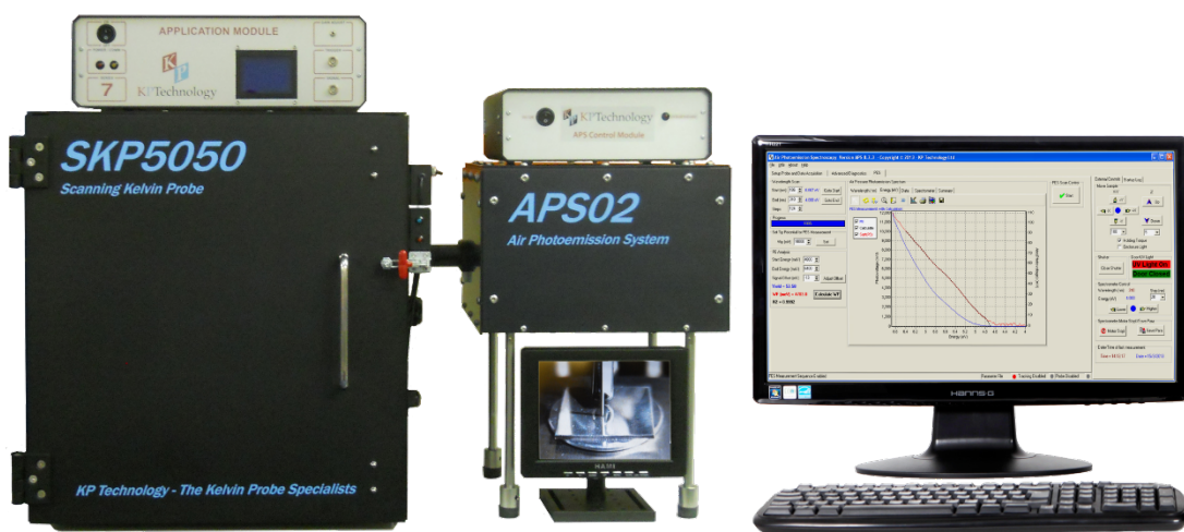
Figure 2.7 Photograph showing Kelvin Probe-Air photoemission spectroscopy set-up, taken from [202].
