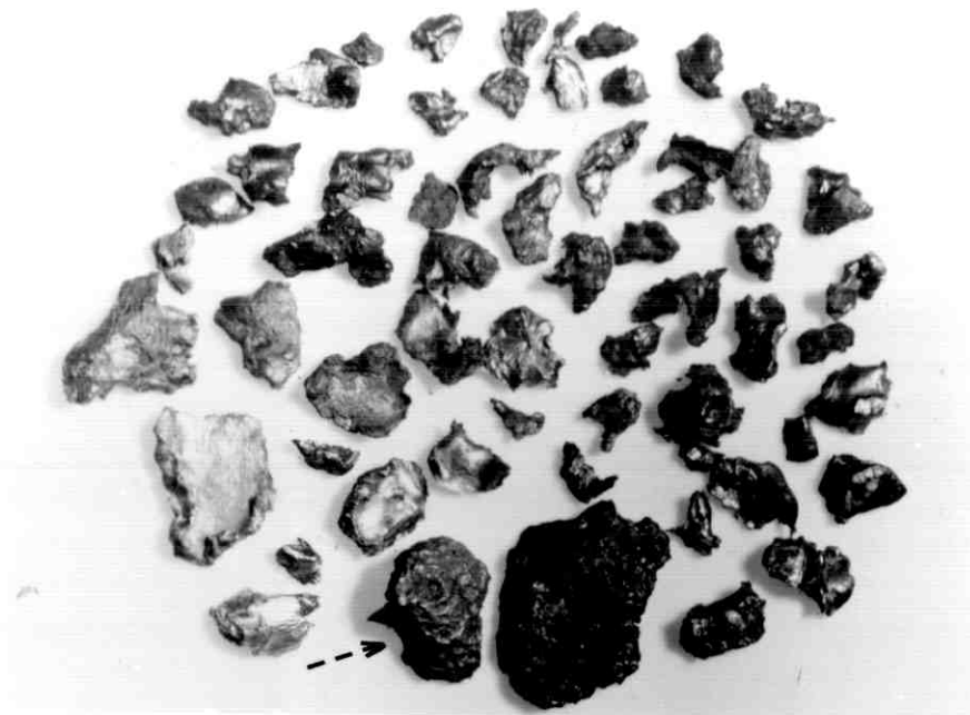
Fig. 3.14 e Fragments of HMX loaded iron (disc indicated)
