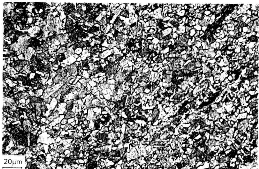
Fig. 4.5 c Recrystallization in HMX loaded copper
