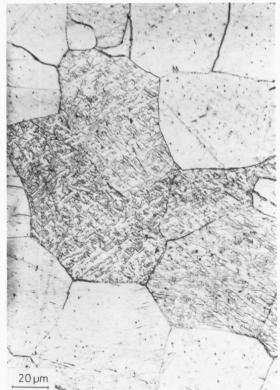
Fig. 4.2 d Darkly etched grains in region corresponding to third hardness plateau (C in Fig. 4.2 e)
