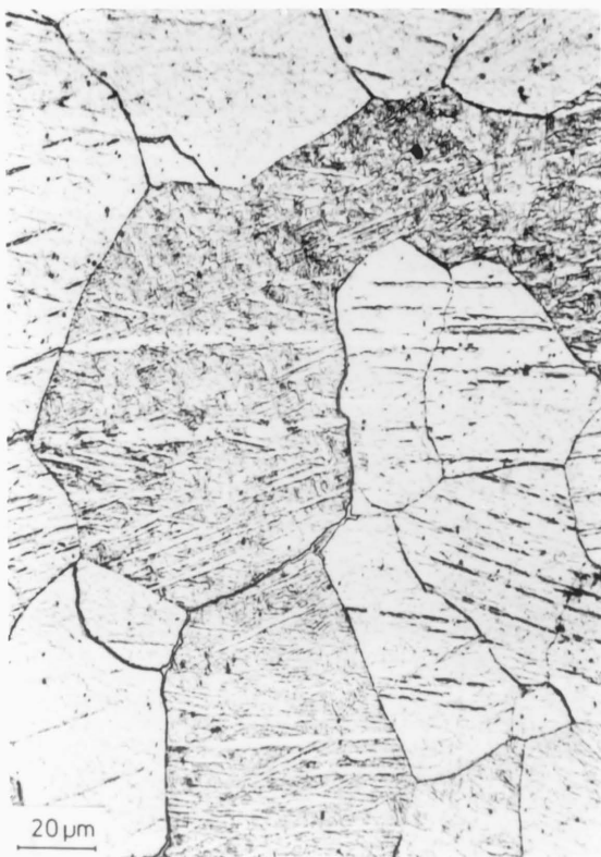
Fig. 4.2 c Heavily twinned and darkly etched grains in region corresponding to second hardness plateau (B in Fig. 4.2 a)
