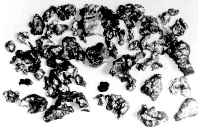
Fig. 3.14 f Fragments of HMX loaded copper (disc destroyed)
