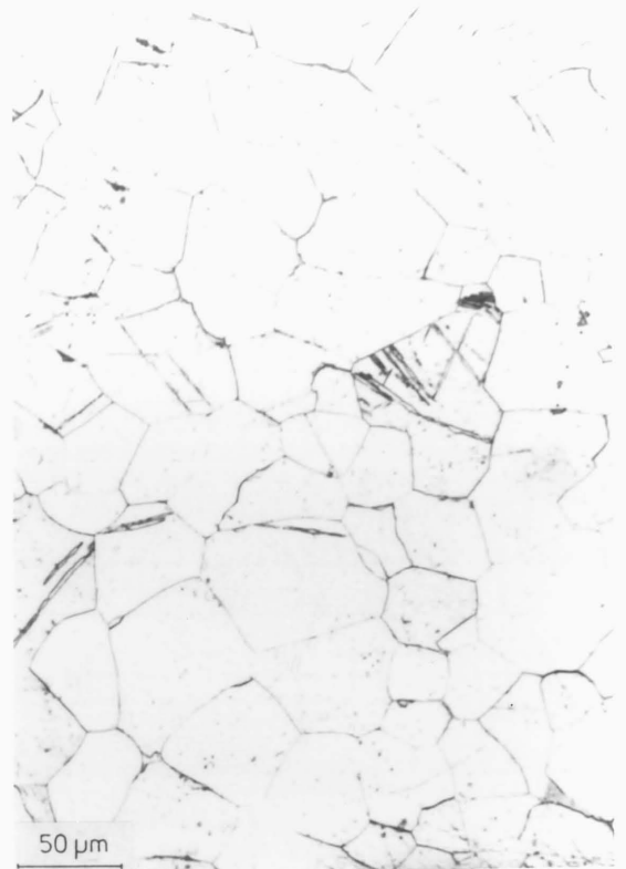
Fig. 4.2 b Onset of twinning (A in Fig. 4.2 a)
