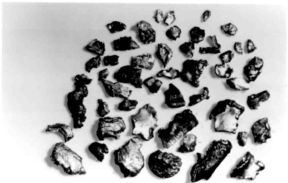
Fig. 3.14 d Fragments of HMX loaded 18/8 steel
