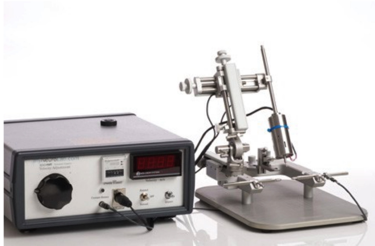
Figure 2.13: The electromagnetic digital CCI device mounted on a stereotactic frame. Photograph taken from Leica MyNeurolab CCI device manual.
