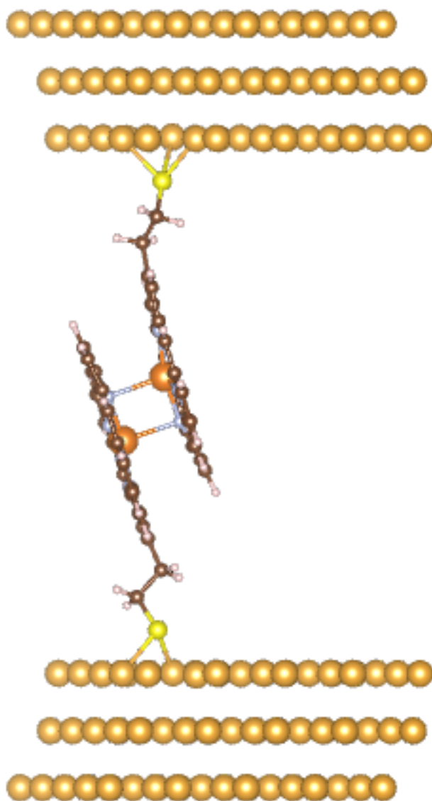
Figure 7.15: The geometry of the porphyrin capacitors. Mg atoms were placed in the center, and the interaction between Mg and N on the other porphyrin molecule stabilizes the geometry, forming a dimer.
