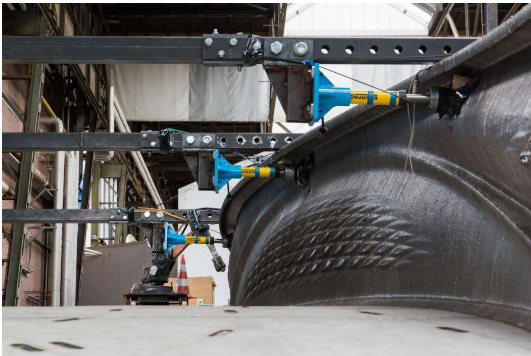
Figure 13: Horizontal load testing of handrails of MX3D bridge
