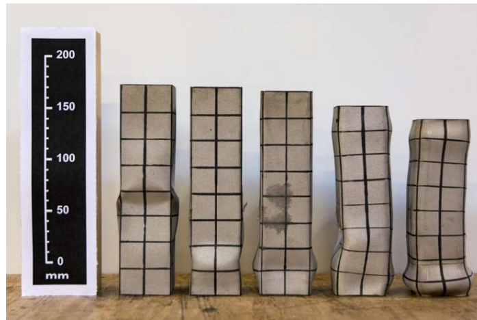
Figure 11: Tested powder bed fusion 3D printed stainless steel stub columns [91]
