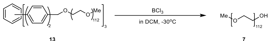
Figure 41. Reaction scheme of the cleavage reaction to yield linear MeO-Eg 112 -OH (mPEG 4967 alcohol, 7).
