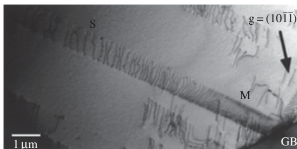
Figure 9. A slip band (comprising mostly \langle a \rangle type slip) developed in creep impinging on a grain boundary (GB), with dislocations of mixed mode (M) close to the GB and screw (S) within the bulk of the \alpha grain [105].
