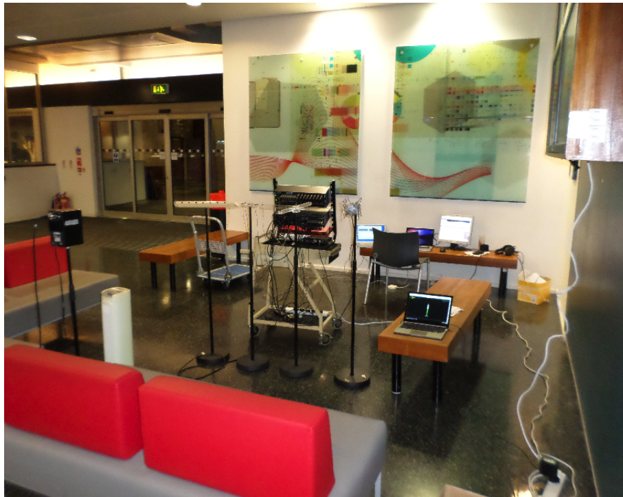
Figure 6.1: Recording session in the Building Lobby before the occupants arrive with microphones in Position 1
