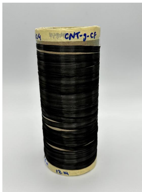
Figure 2: An example spool of CNT-g-CF used to determine the weight percentage of carbon nanotubes on the fiber after synthesis on open CVD line (12 m).
