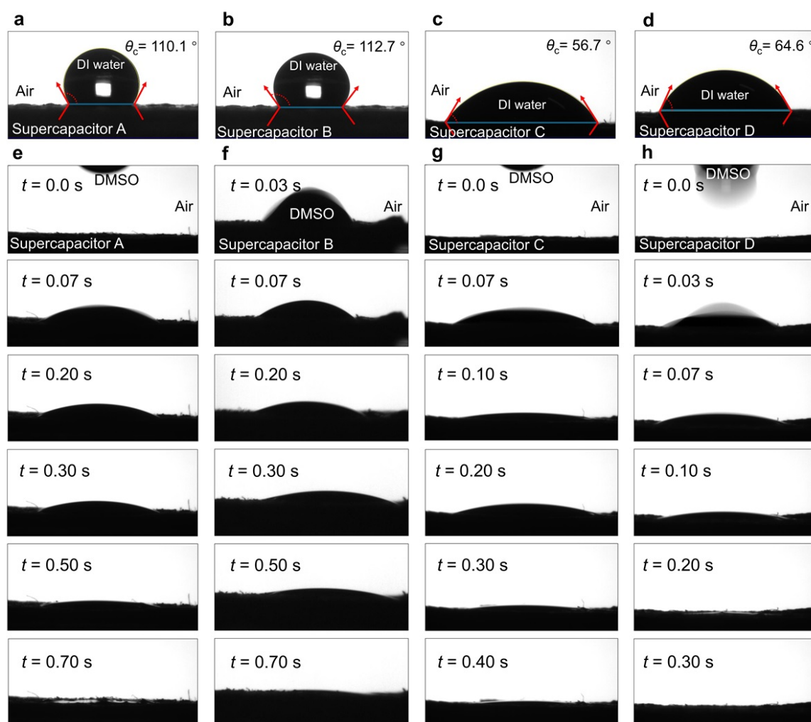
Fig. B.4 The wettability of supercapacitor electrodes using different materials. Water \theta_c tests of supercapacitor A (a), B (b), C (c), and D (d); and the absorption of DMSO into the textile supercapacitor of supercapacitor A (a), B (b), C (c) and D (d).
