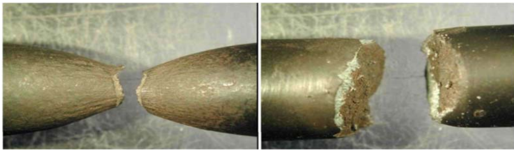
Figure 5: Fracture surface of Grade 91 crept specimen after (a) 100 hours at 550°C and (b) 20,014 hours at 650°C [45]
