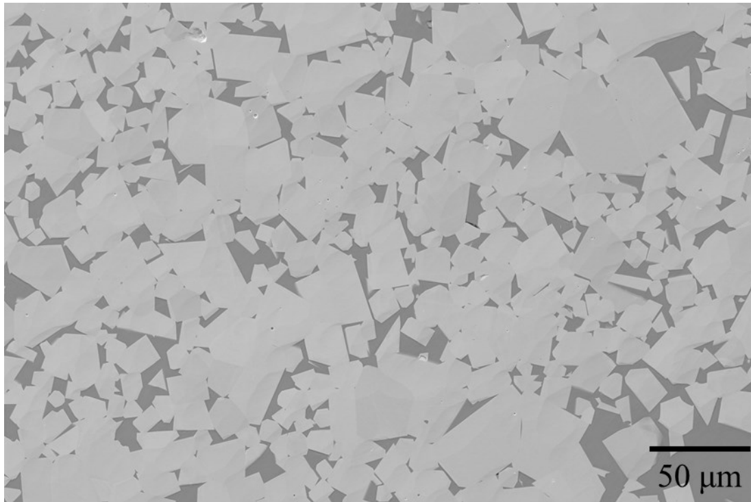
Figure 1.5: SEM micrograph of a WC-10wt%Co specimen in SE mode. Brighter and darker regions are WC grains and Co ligaments respectively.
