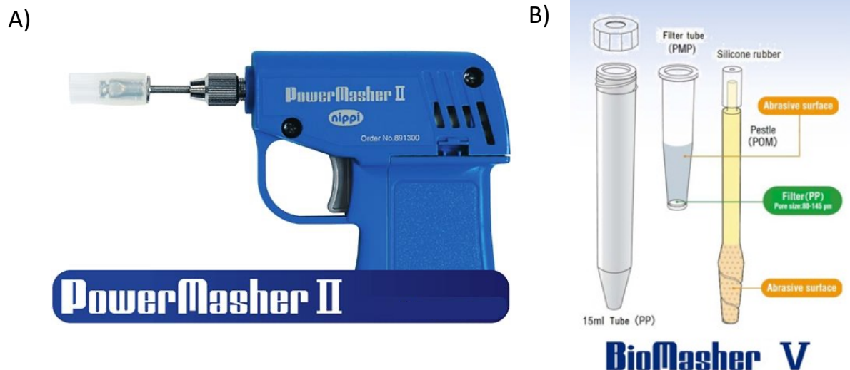
Figure 5.1. Commercially available portable tissue homogenisation devices. The handheld battery-operated electric homogeniser, the PowerMasher II, including a rubberised pestle holder to the rapid change of homogenisation pestles (A). The BioMasher V is a sterile, single-use homogenisation system consisting of a plastic pestle with a textured tip encapsulated into an inner filter tube (80-145 µm pore size) which filters homogenised tissue into the supplied 15 mL centrifuge tube (B). Image used with the permission of the copyright holder, nippi-inc.
