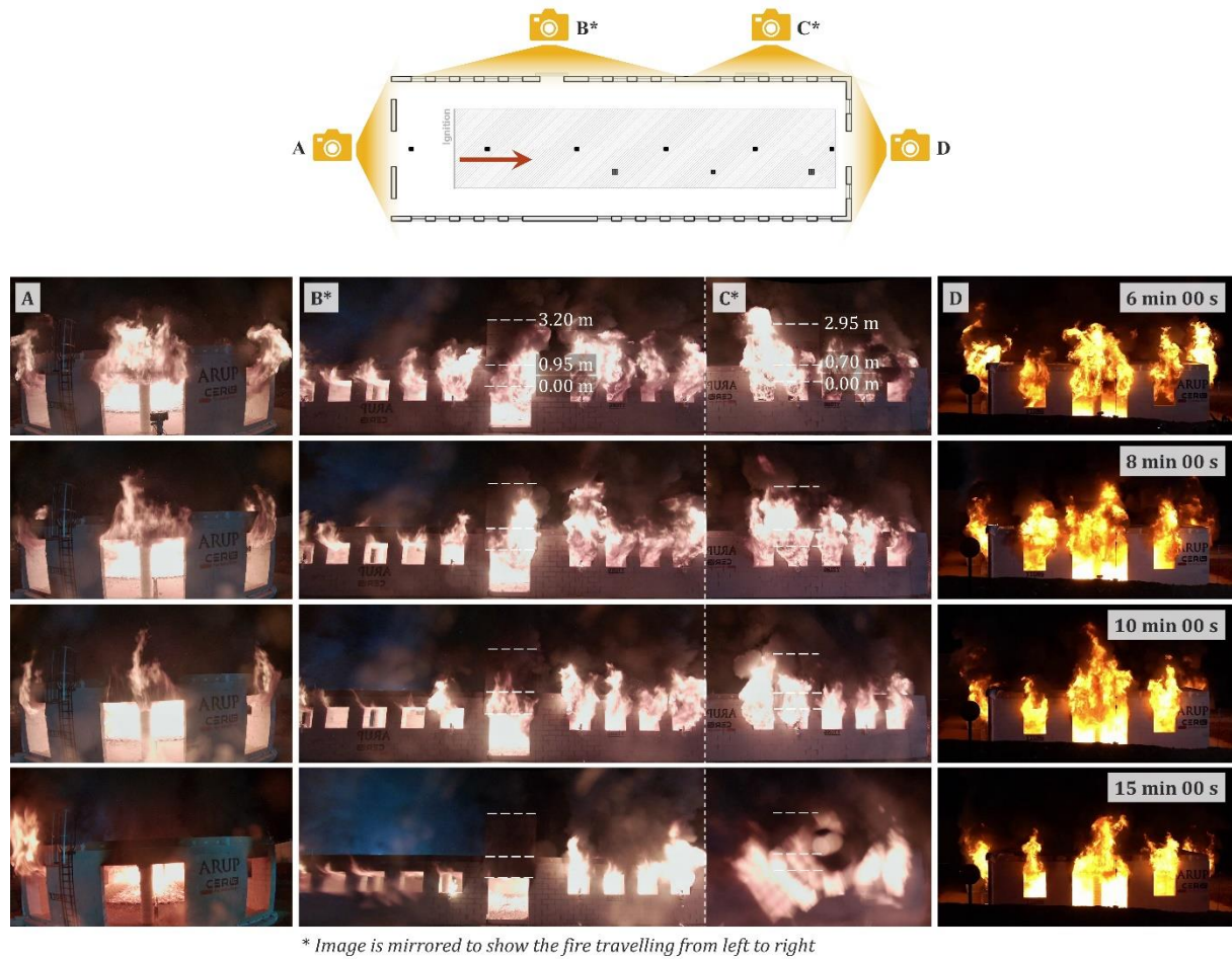
Figure 20. Selection of images captured during the experiment showing the size and progression of the external flaming observed during the peak burning period. Earlier timesteps are shown in Figure 7. The times annotated are the duration since ignition.
