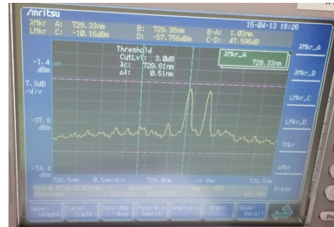
(b) Output of slave laser with imperfect injection lock.
