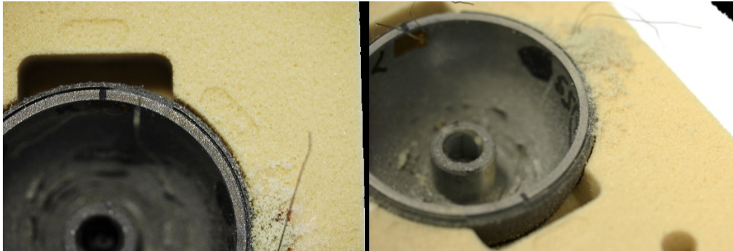
Figure 5.3.4: An acetabular cup in seated in low density bone with 10 strikes of high velocity and high mass. A large amount of bone substitute debris has gathered around the cup rim. In addition a clear gap is visible between the cup and bone.
