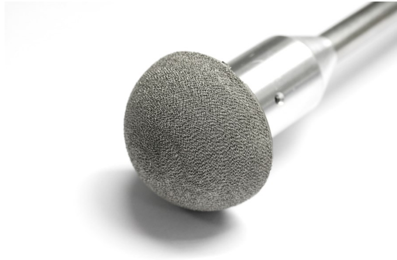
Figure 4.2.2: Custom acetabular cup with surface finish resembling that of typical plasma-spraying
