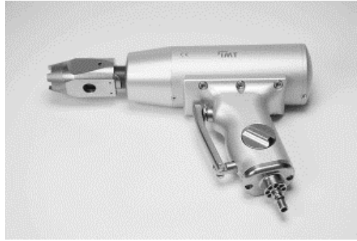
Figure 2.5.1: Pneumatic oscillatory impaction tool: The 'Woodpecker' by IMT 204
