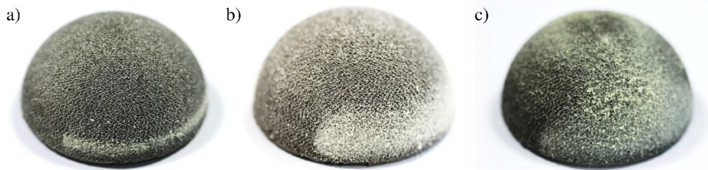
Figure 4.3.6: Residue synthetic bone debris following implantation at: a) 1.4 J b) 6.8 J c) 14.4 J. An increase in energy corresponds with an increase in debris coverage, from the rim (at low energy) to the pole (at high energy)
