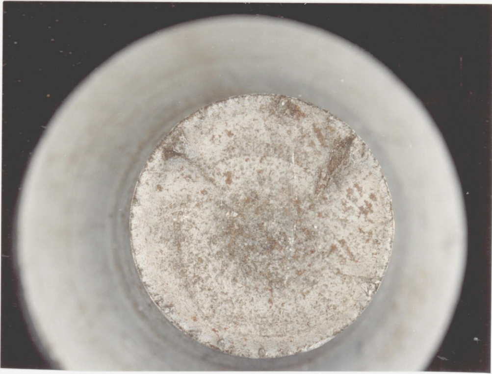
Figure 6.29 unnotched Failed cross-section of failed Specimen No. 5
