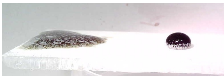
FIGURE A.5: Droplet of water resting on a surface coated with TiO 2 super-hydrophobic paint after 3 hours the preliminary experiment was initiated
