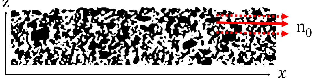
FIGURE 4.2: Example of binarised slice of porous sample. The X-ray tomography method produces a sequence of slices of the sample, showing the internal structure of the porous material. The black areas are the solid surface, and white areas are the porous channels.
