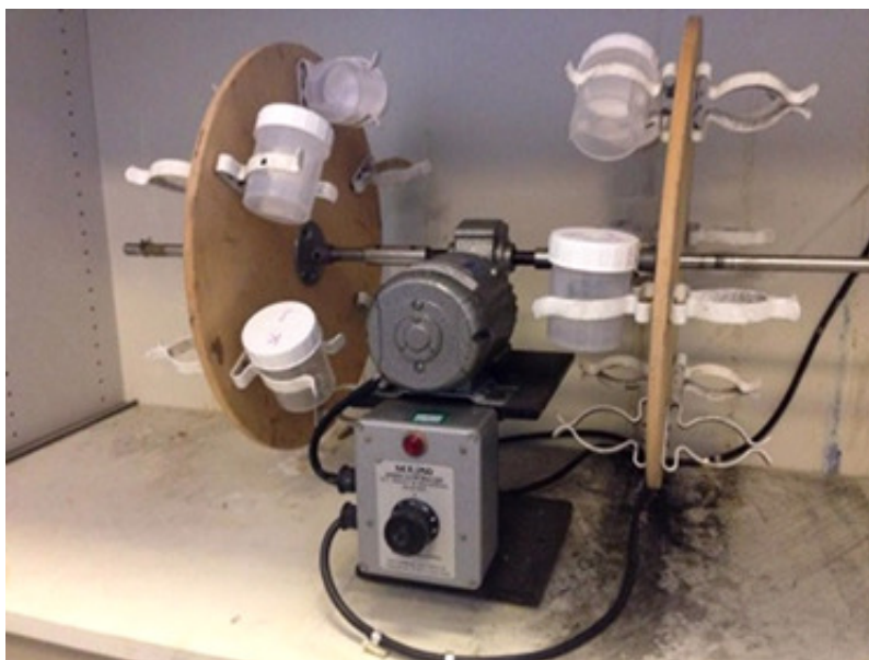
FIGURE 2.3: Plastic containers placed in an equipment with wooden discs attached to the side. The wooden discs rotate, preventing stagnation of the water in the plastic containers. The motion of water in the plastic containers contributed to the depletion of air trapped on the surface of the super-hydrophobic coatings.
