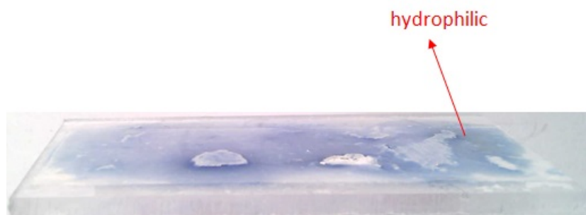
FIGURE A.3: Droplet of water resting on a surface coated with PSA after 6 hours the preliminary experiment was initiated
