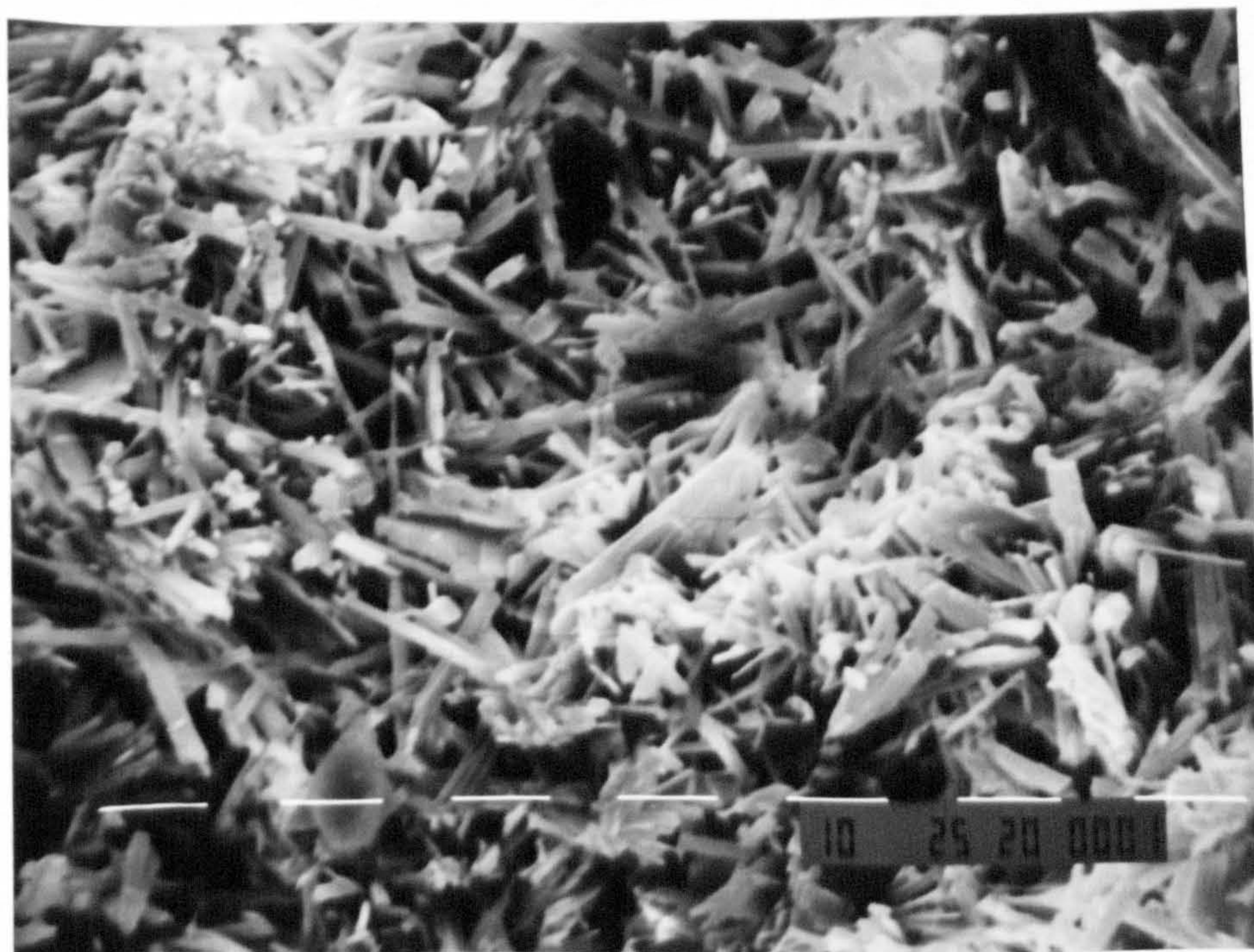
Plate 4.6: Scanning electron micrograph, at x1000, of the microstructure of the fully set plaster from Guilini plaster (W/P ratio = 0.6).
