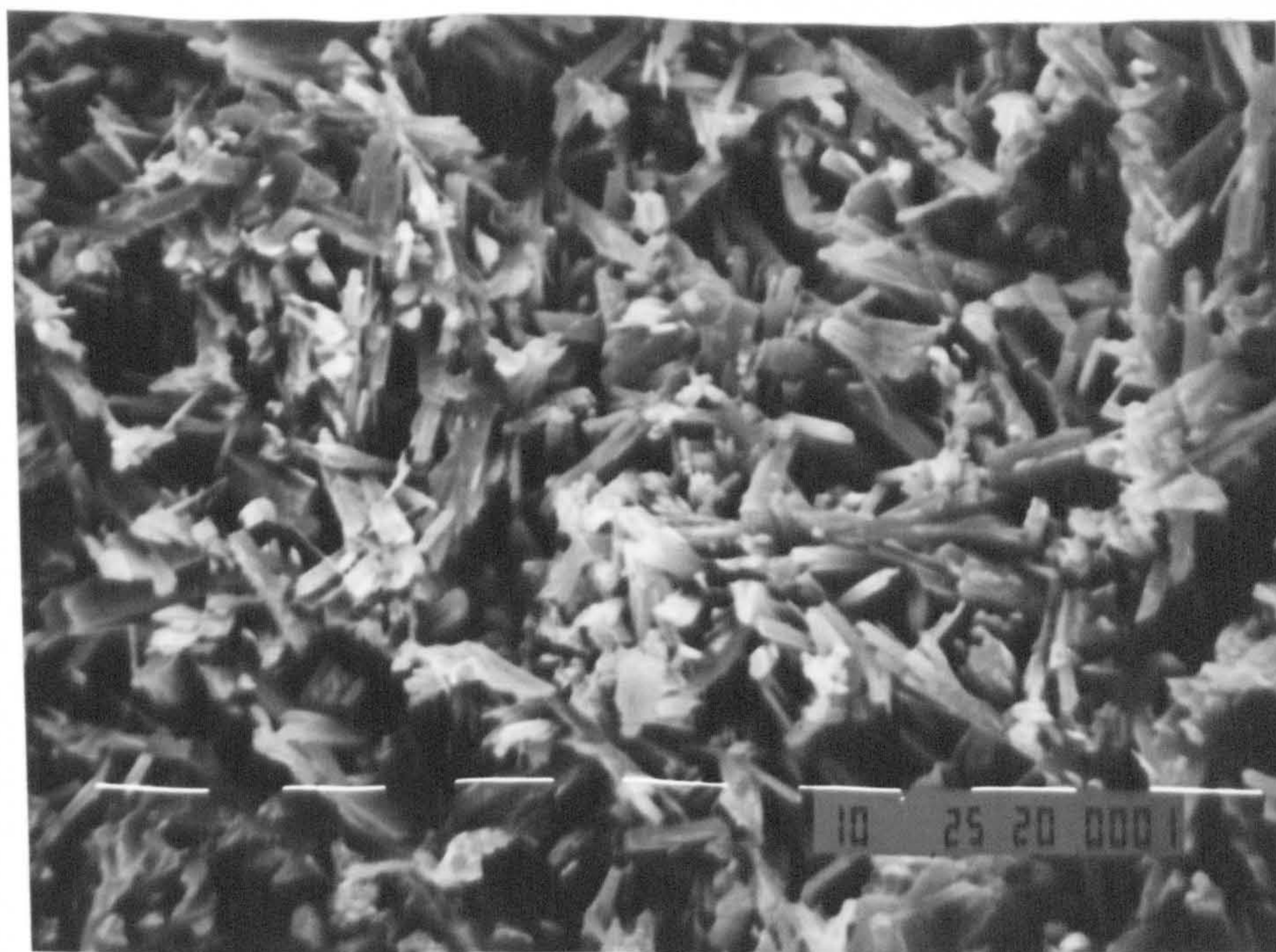
Plate 4.3: Scanning electron micrograph, at x1000, of the microstructure of the fully set plaster from British Gypsum \alpha (W/P ratio = 0.6).
