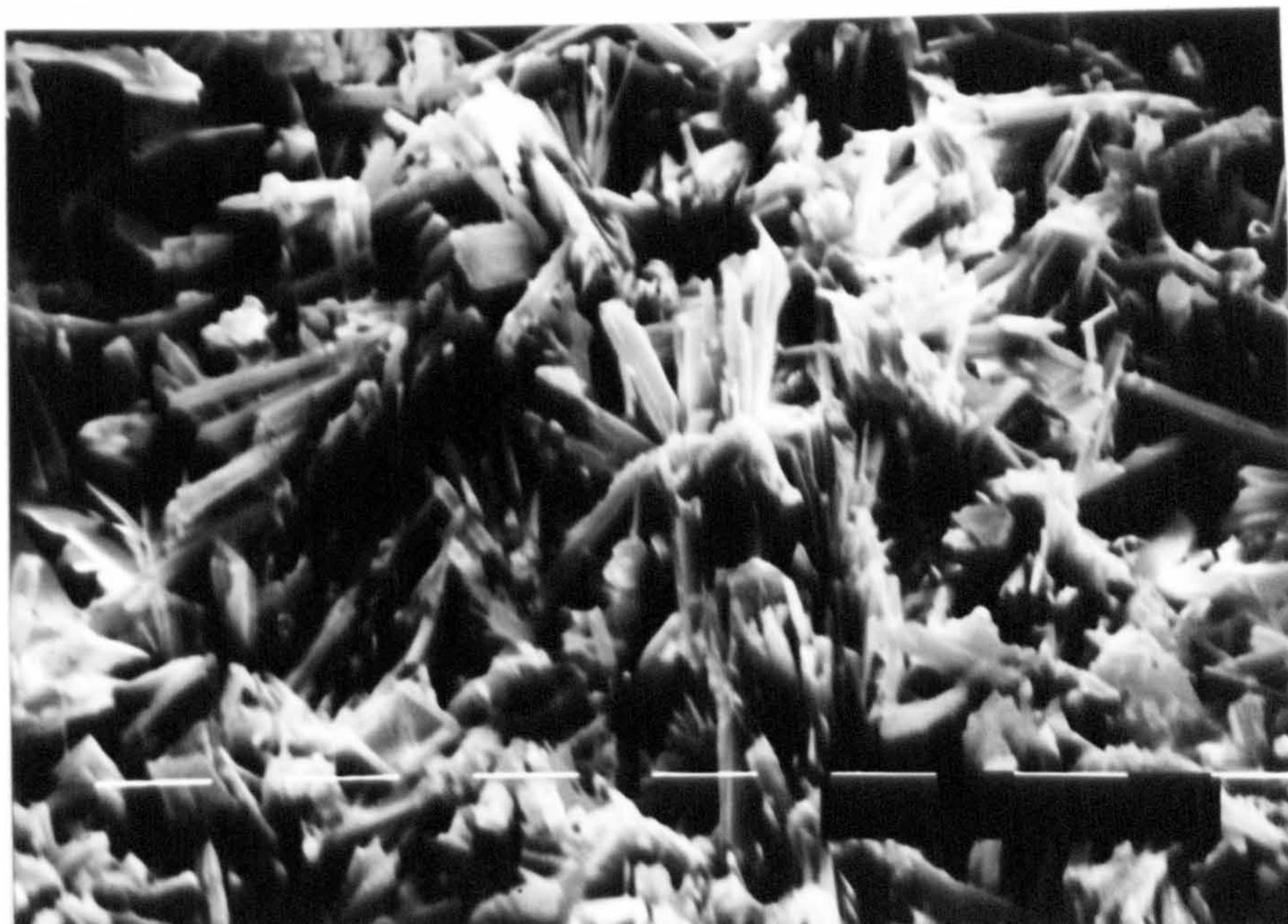
Plate 4.30: Scanning electron micrograph, at x1000, of the set plaster from 50wt% \alpha /50wt% \beta -hemihydrates (W/P ratio = 0.56).
