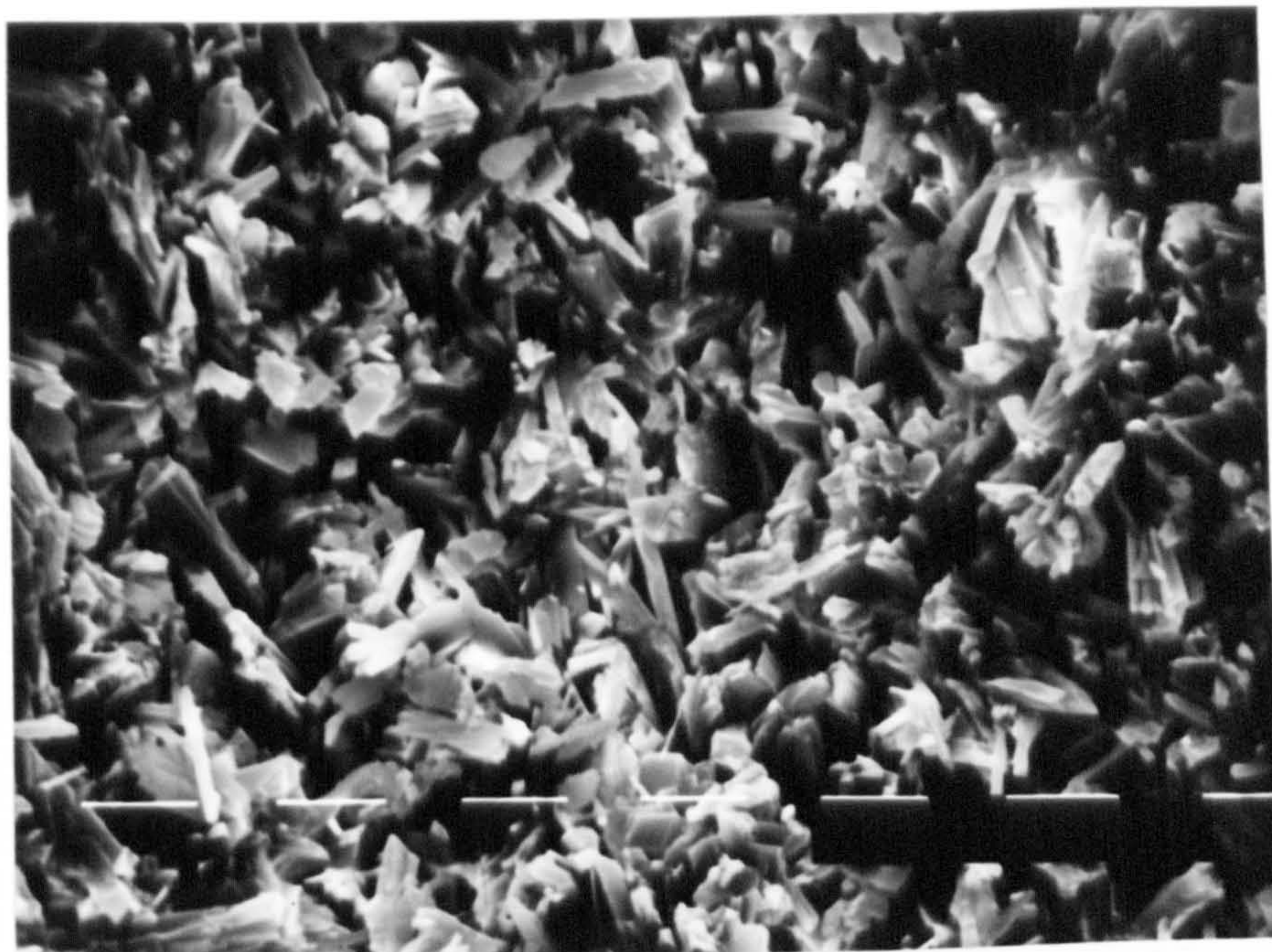
Plate 4.28: Scanning electron micrograph, at x1000, of the set plaster from 100wt% \alpha -hemihydrate. (W/P ratio = 0.45).
