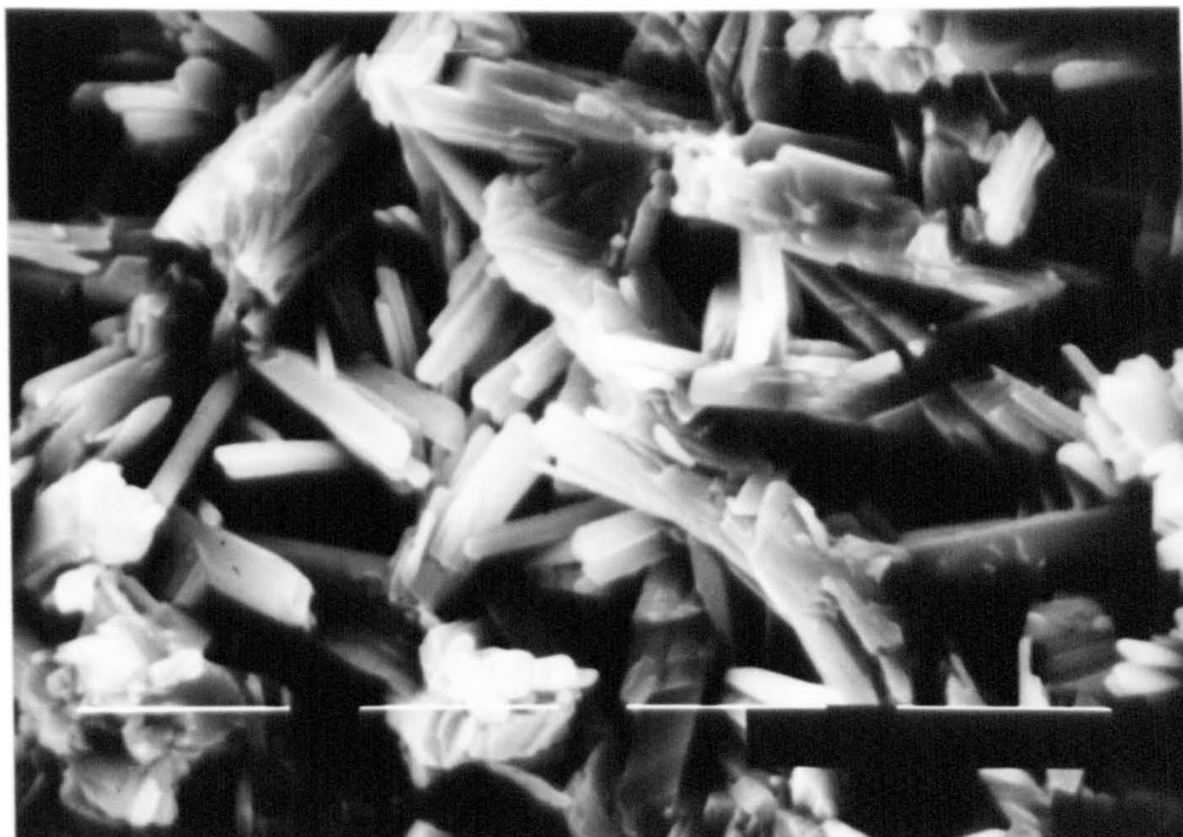
Plate 4.24: Scanning electron micrograph, at x2000, of the set plaster from \alpha -hemihydrate plus 1wt% K_2SO_4 (W/P ratio = 0.6).
