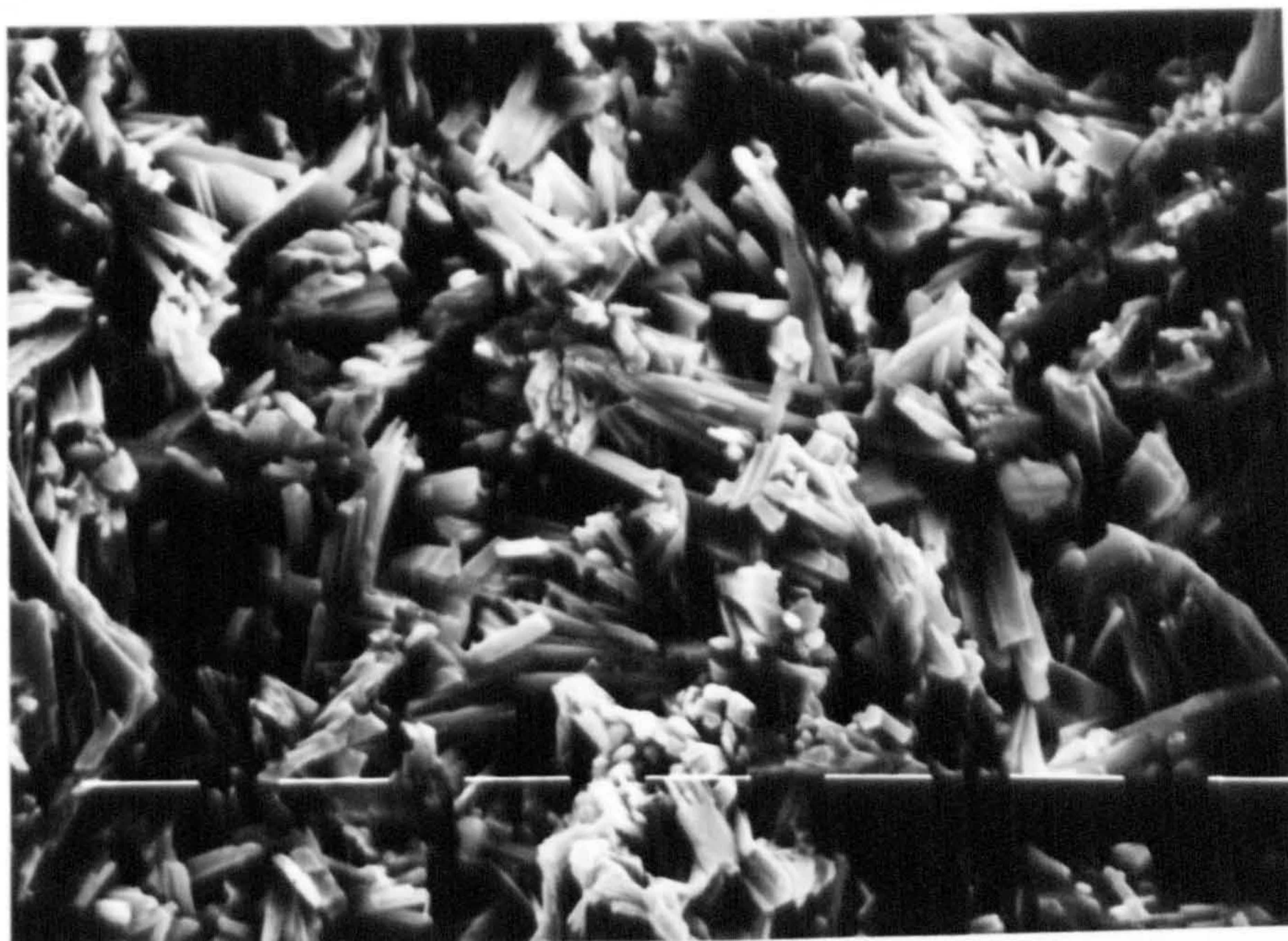
Plate 4.26: Scanning electron micrograph, at x1000, of the set plaster from \alpha -hemihydrate (50g) plus \text{Ca}(\text{OH})_2 (0.22g) and \text{KHSO}_4 (0.79g) (W/P ratio = 0.6).
