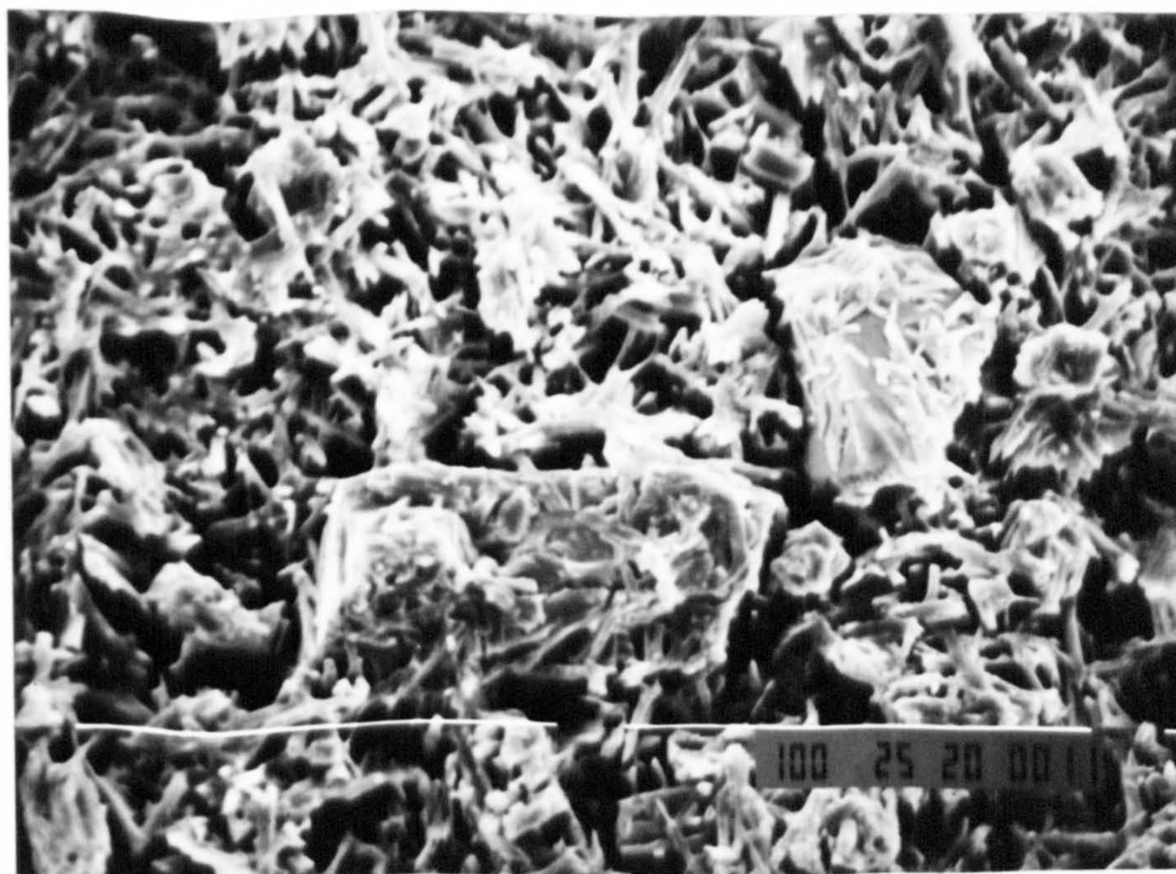
Plate 4.7: Scanning electron micrograph, at x500, of the solid phases present in a partially reacted mixture of \alpha -hemihydrate and water after 45 mins. (W/P ratio = 0.6).
