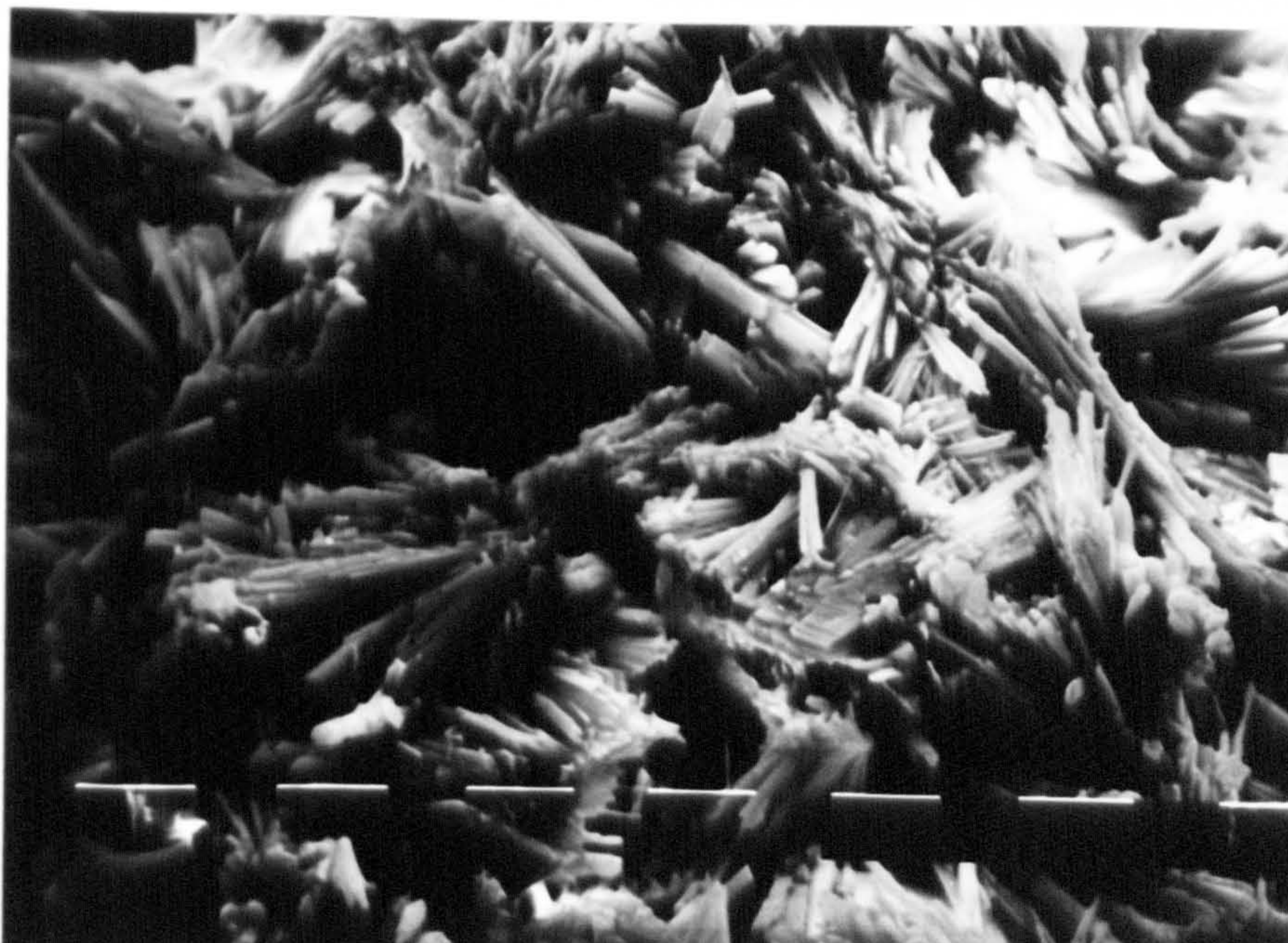
Plate 4.32: Scanning electron micrograph, at x1000, of the set plaster from 100wt% \beta -hemihydrate (W/P ratio = 0.68).
