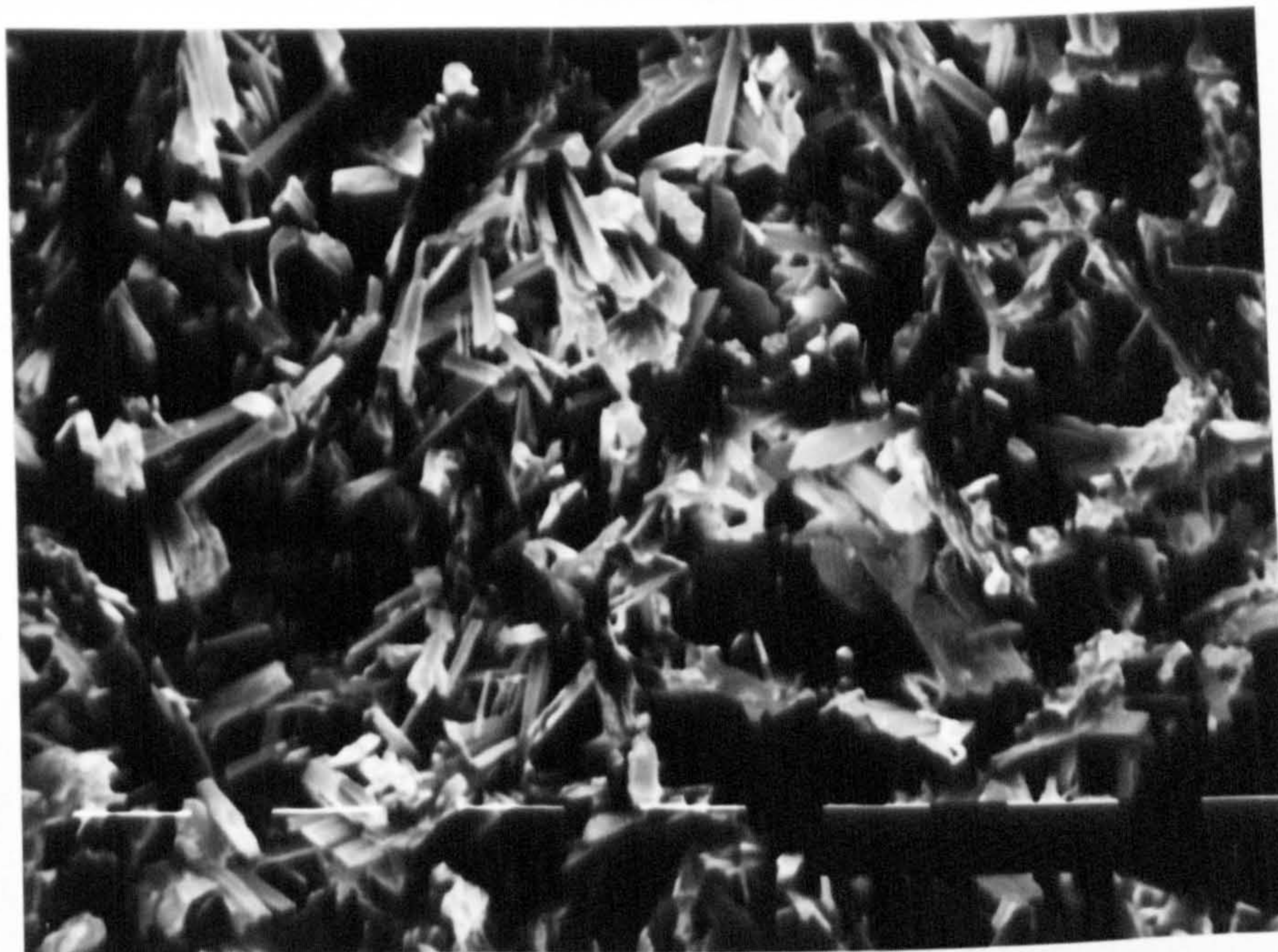
Plate 4.29: Scanning electron micrograph, at x1000, of the set plaster from 75wt% \alpha /25wt% \beta -hemihydrates (W/P ratio = 0.51).
