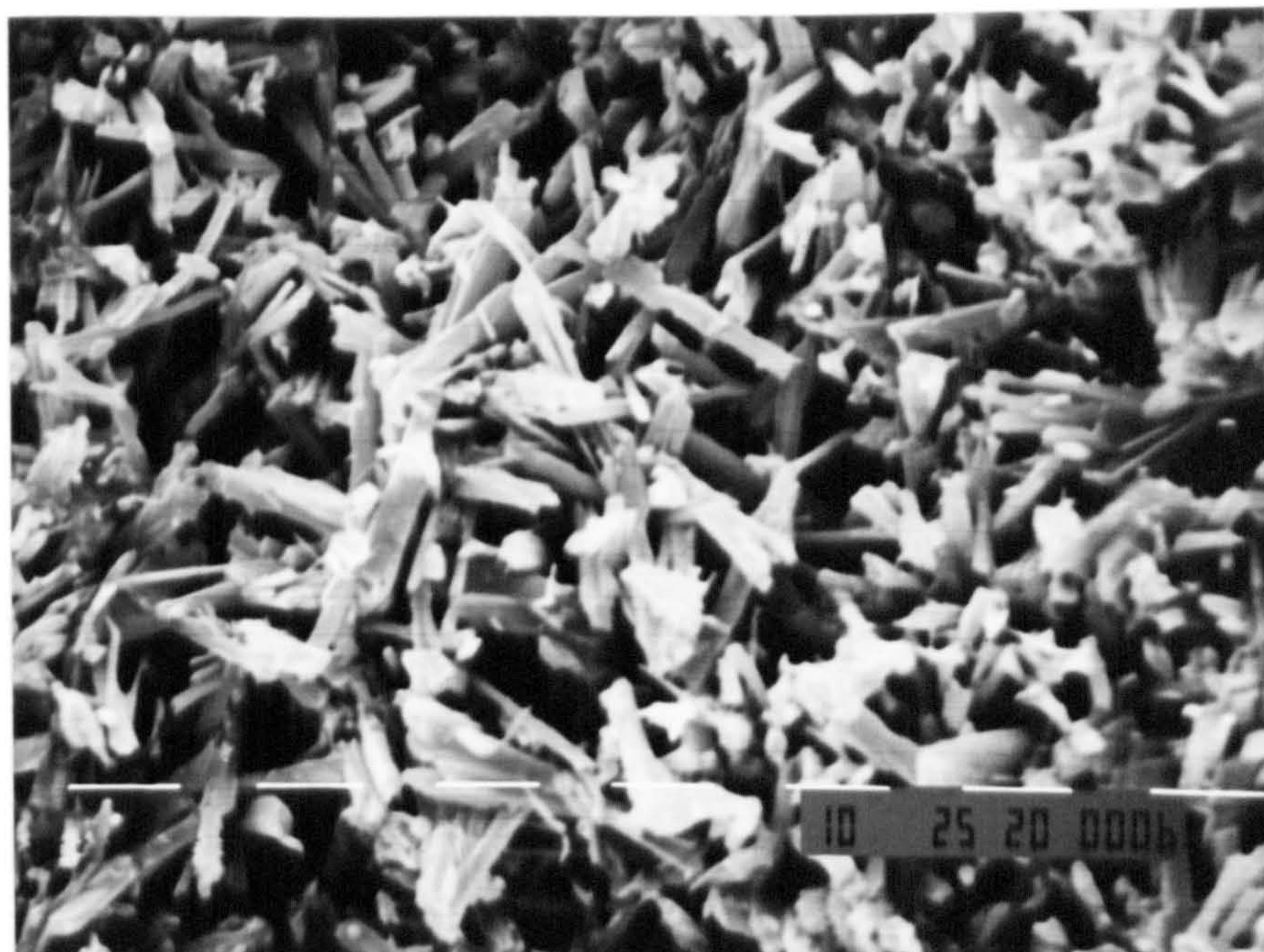
Plate 4.16: Scanning electron micrograph, x1000, of the microstructure of set plaster from 90wt% \alpha -hemihydrate/10wt% \alpha -soluble anhydrite (W/S ratio = 0.6).
