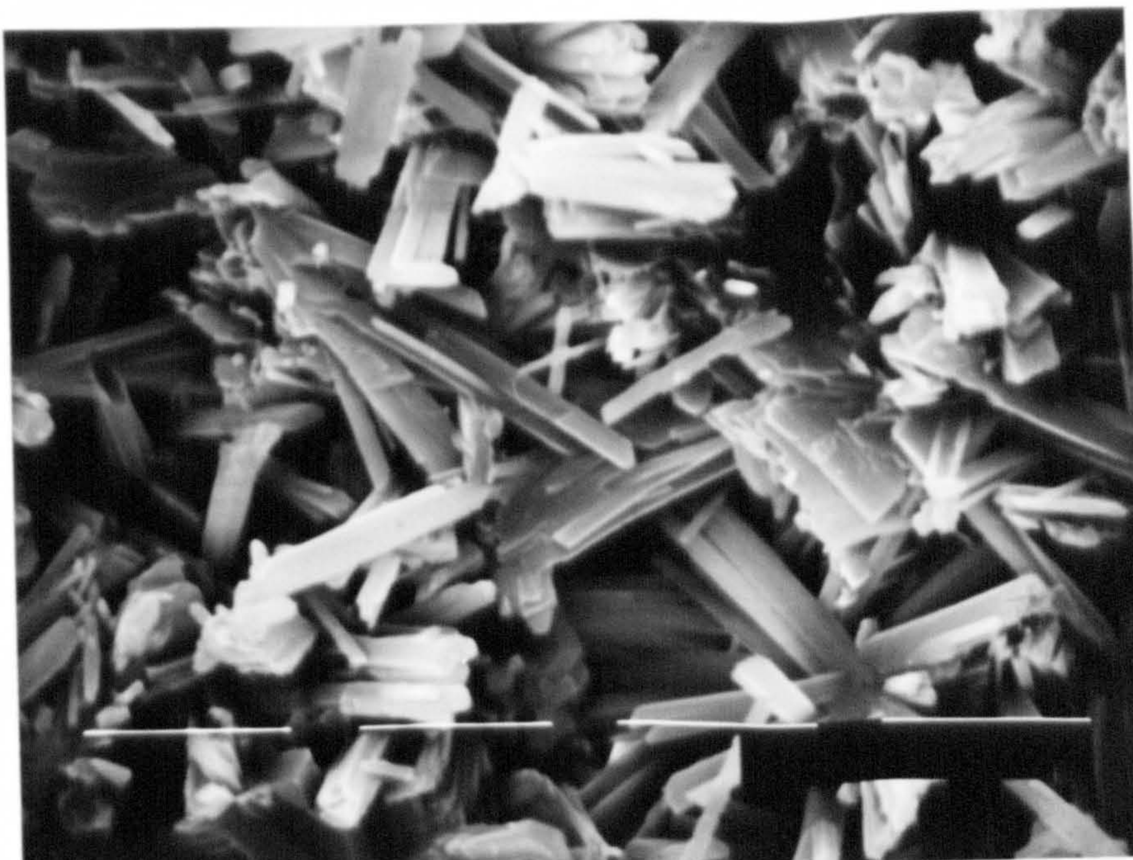
Plate 4.22: Scanning electron micrograph at x2000, of the set plaster from \alpha -hemihydrate (W/S ratio = 0.6).
