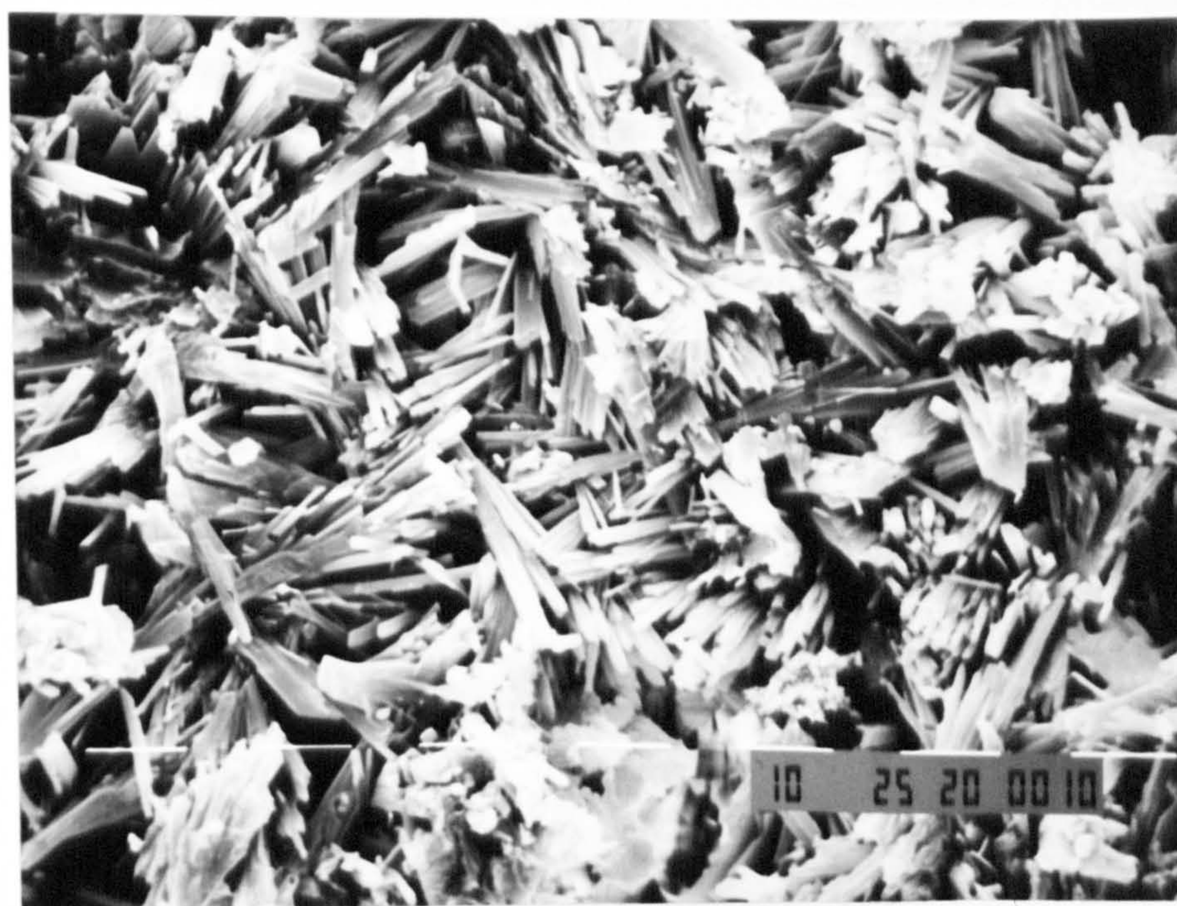
Plate 4.17: Scanning electron micrograph, x1000, of the microstructure of set plaster from 90wt% \beta -hemihydrate/10wt% \beta -soluble anhydrite (W/S ratio = 0.6).
