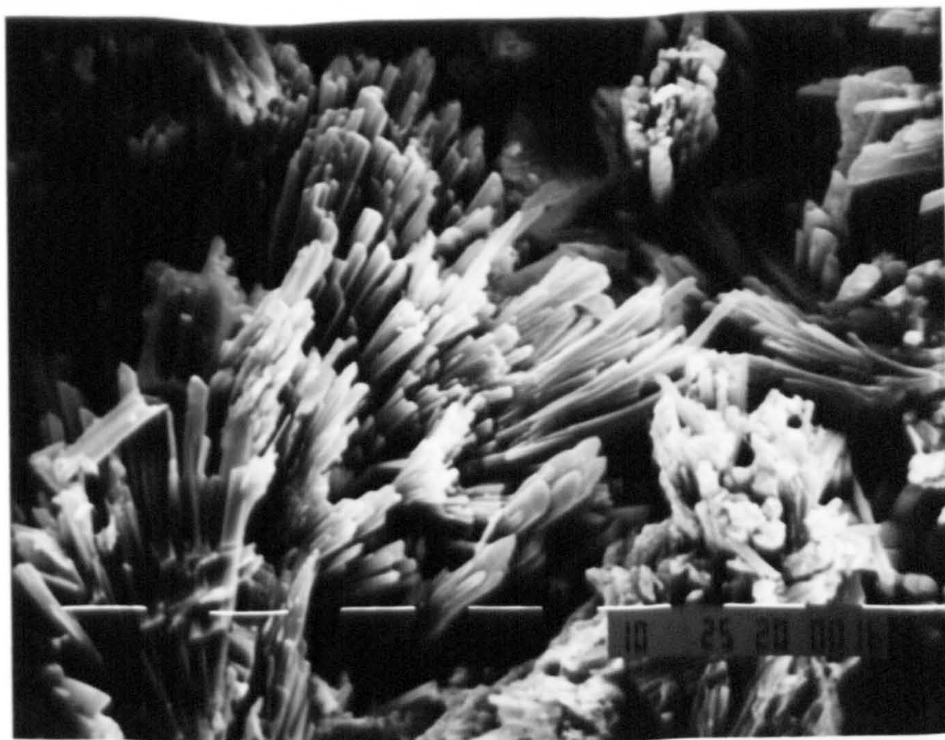
Plate 4.15: Scanning electron micrograph, at x1000, of the solid phases in the ' \beta '-soluble anhydrite/saturated dihydrate solution reaction mixture after 1 hour.
