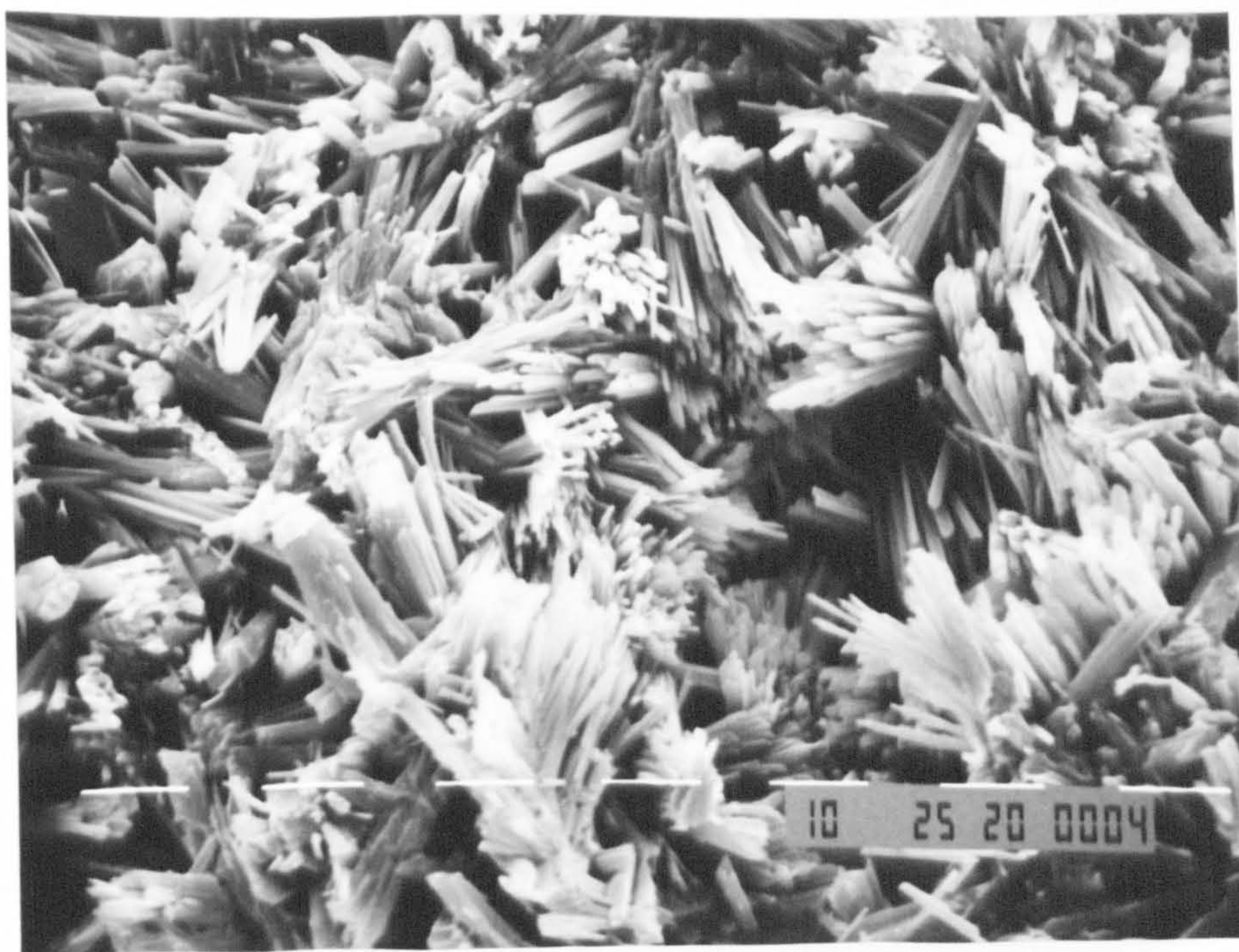
Plate 4.4: Scanning electron micrograph, at x1000, of the microstructure of the fully set plaster from British Gypsum \beta (W/P ratio = 0.6).
