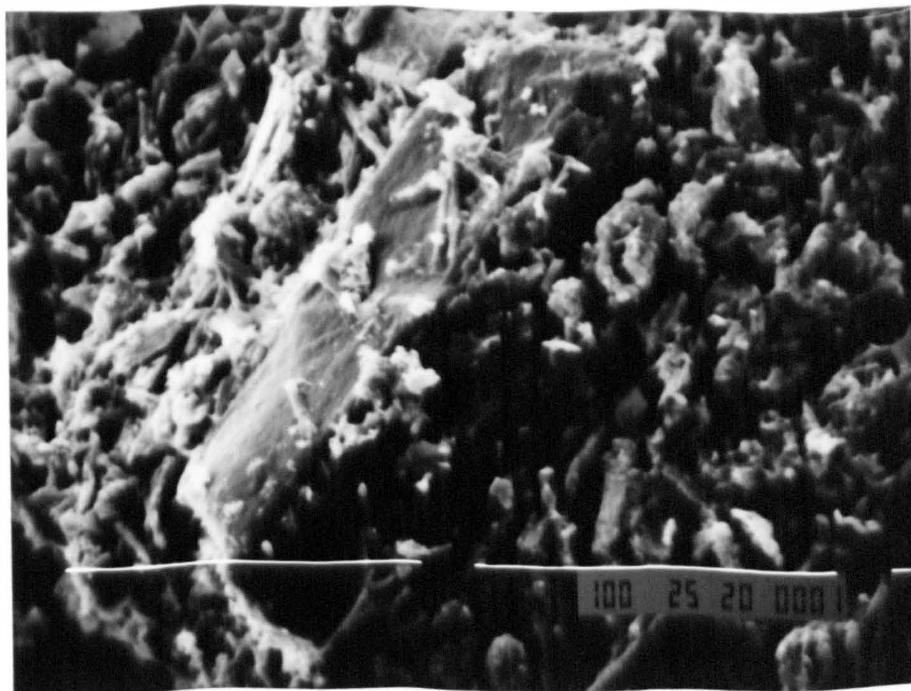
Plate 4.9: Scanning electron micrograph, at x500, of the solid phases present in a partially reacted mixture of \beta -hemihydrate and water after 45 mins. (W/P ratio = 0.6).
