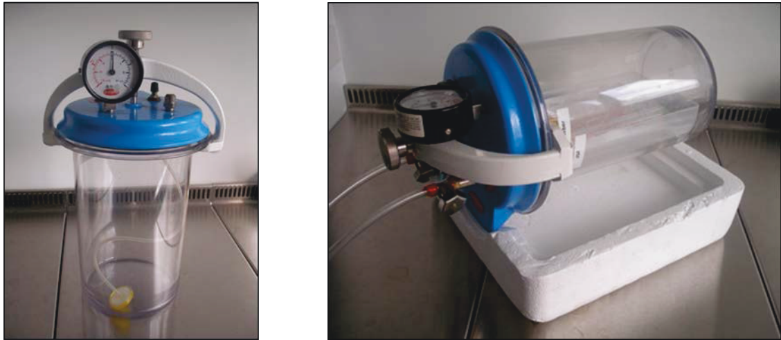
Figure 10: Oxoid hypoxic chamber. Prior to each incubation, the chamber was secured in a horizontal position. Plates were loaded along with a T-25 flask containing sterile water to ensure sufficient humidification. After sealing, the chamber was evacuated (-0.6 Bar) and filled with a hypoxic gas mixture (1% O 2 , 5% CO 2 ) (repeated 3x as per manufacturer's instructions) and placed in a standard incubator set to 37°C.
