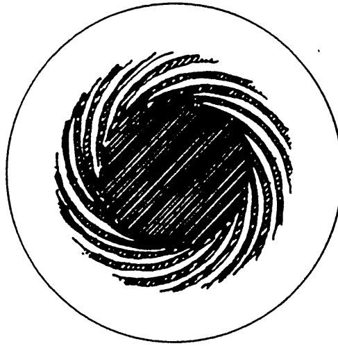
Fig. 23 Schematic diagram of the transition from the central, laminar flow region (shaded zone), through the transition zone, where there are standing waves, to the turbulent zone.
