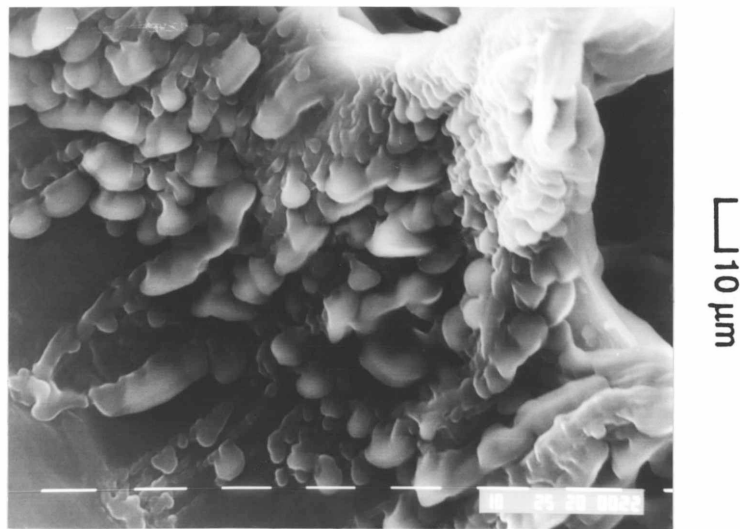
Fig.4.60 Micrograph of the fracture morphology at the notch tip
