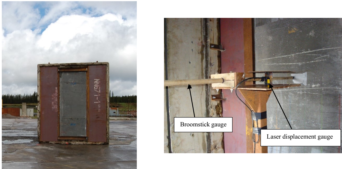
Figure 2-2 – Sensor arrangement for fibre-reinforced concrete panel tests conducted by Barnett et al. (Left) External view of panel in test cubicle. (Right) Pre-test image of ‘broomstick’ and laser gauges. (Author’s photographs)
