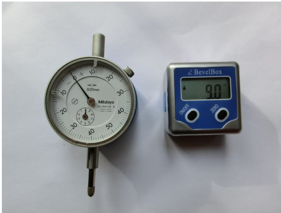
Figure 3-25 – Analogue dial gauge sensor (left) and digital protractor (right)
