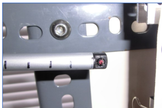
Figure 7-4 – Photograph showing the 'shear pin' in the end of the actuator (left) and a close-up image of the 'shear pin' (right)
