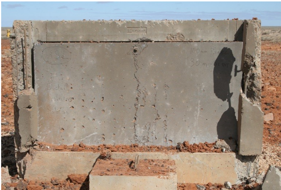
Figure 2-1 – Image of one of the UHSPC panels tested by Ngo et al (Author's photograph)
