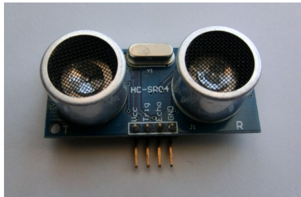
Figure 3-15 – Simple ultrasonic distance measuring sensor
