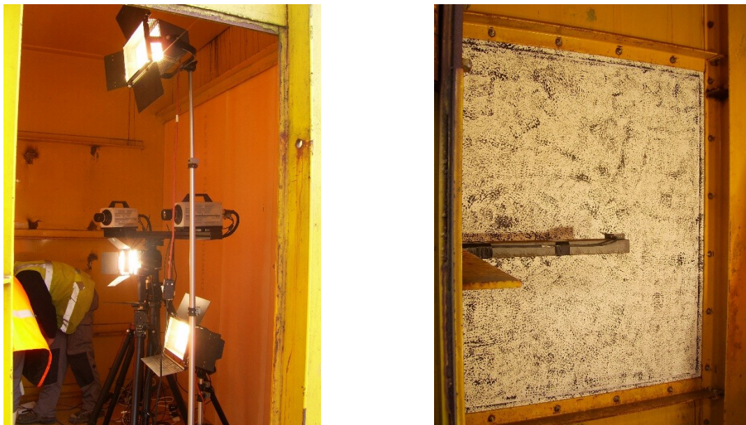
Figure 2-6 – Test arrangement for DIC laminated glass deflection tests conducted by Hooper. (Author’s photographs)
