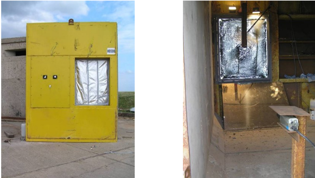
Figure 2-4 – Test arrangement for laminated glass deflection tests conducted by Stephens. (Left) Front of test cubicle showing glass pane with aluminium foil facing. (Right) Rear view of glass pane post-test showing HSV camera and mirror arrangement. (Author’s photographs)
