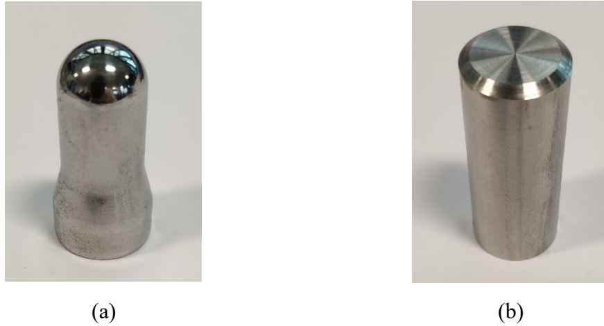
Figure A-1. Illustrations of: (a) the hemispherically-headed (RNS) steel and (b) the flat-ended steel (FFS) impactor with a 45° chamfer on the edge to the flat-ended cylindrical section.
