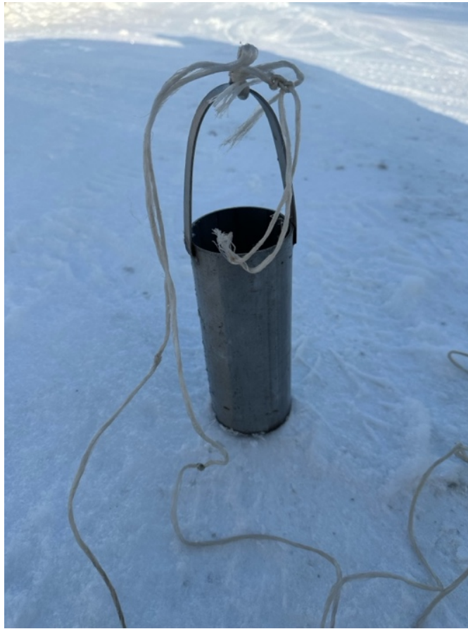
Figure 3.1: A stainless-steel core sampler.
