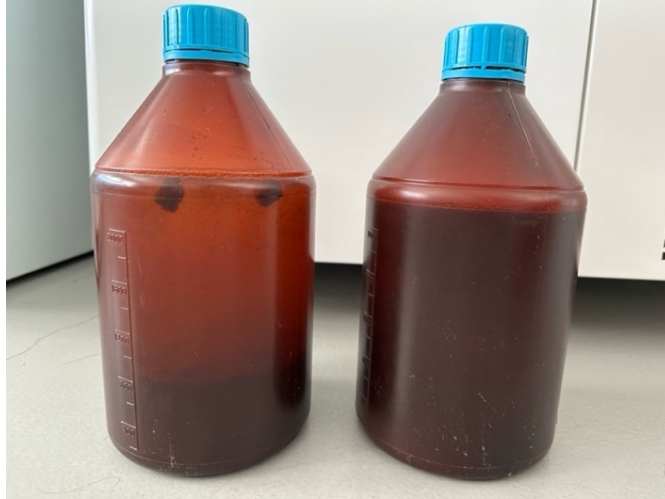
Figure 3.3: Laboratory-scale reactors filled with inoculum.
