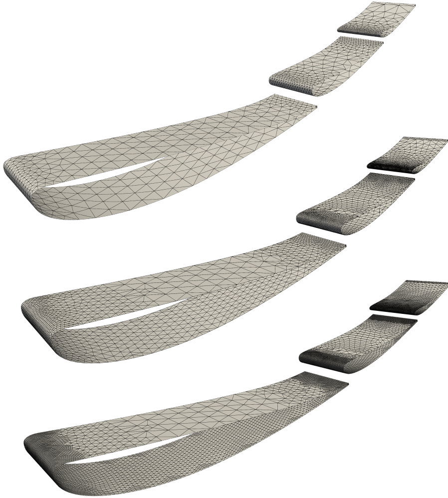
Figure 9.4: The high-order surface mesh of the initial, h-adapted and hh-adapted hybrid meshes based on the time-averaged Q-criterion. Please note the uniform refinement on the suction side of the wings and the lack of refinement on the pressure side of the mainplane and the first flap.
