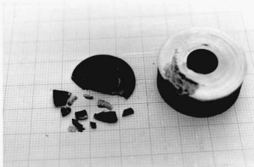
Plate 6.8 Failure of die and specimen brought about by excessive heating and a long contact time. There appears to have been some alloying of the two materials which caused both of them to become unusually brittle in the cold conditions. The failure occurred when separation was attempted.
