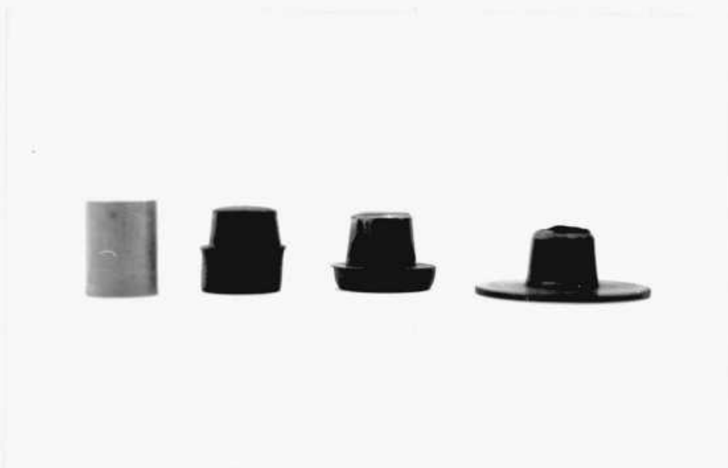
Plate 6.6 Some stages in forming a billet of diameter 25.4 mm with profile dies. The billets have the same volume as those in Plate 6.5
