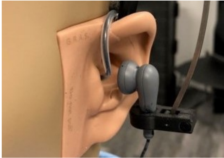
Figure 4.1: Custom floating headphones (Sennheiser MX475) and binaural microphones (Brüel and Kjær 4101-B) mounted on KEMAR head and torso simulator.
