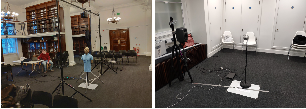
Figure 6.3: The two measured rooms. (Left) The library is shown during a BRIR measurement. (Right) The trapezoid is shown during a RIR measurement.
