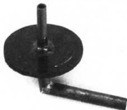
Tube for axial sample injection. (Disc replaces quartz window)
