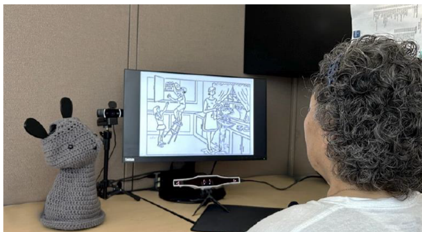
Figure 5.8: Experimental setup during a picture description task. The figure shows a participant interacting with Blossom while looking at the screen with the Cookie Theft picture displayed. Photo used with consent.
