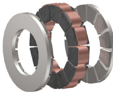
Figure 1.5 Yokeless and segmented armature machine, from [18]
