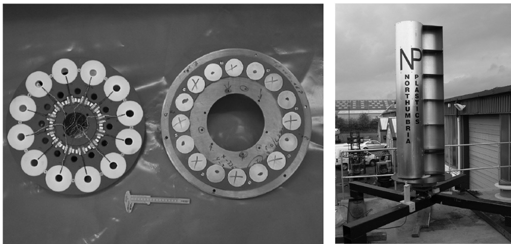
Figure 1.4 Axial flux generator (left), wind turbine application (right), from [12]
