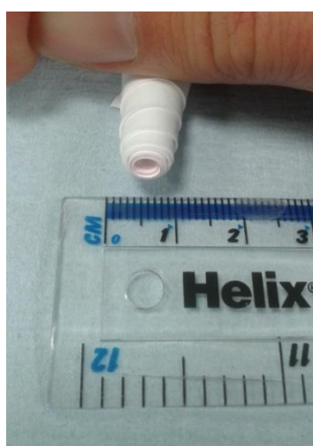
Fig 7.4 Flexible porous films rolled up to a cylinder with a diameter less than 10 mm.
