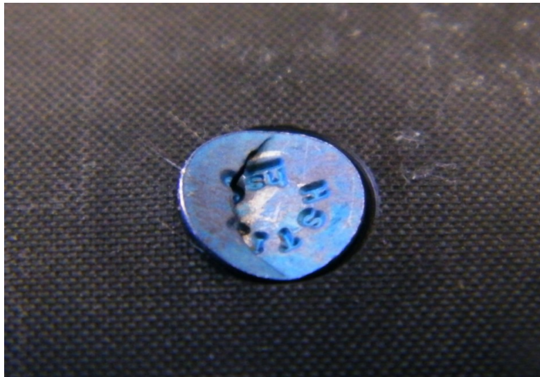
Figure 3-15. Cracked countersunk bolt head in single-lap composite joint after tensile test.
