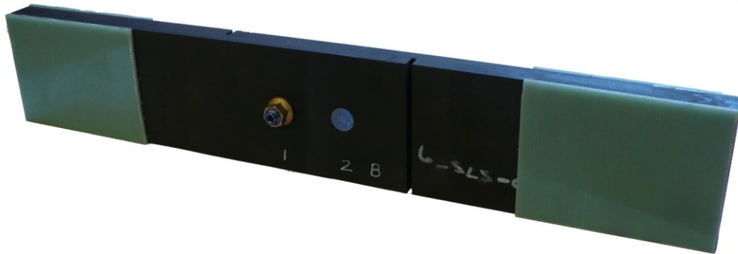
Figure 4-1. Specimen of a composite bolted joint for the fatigue single lap shear test.
