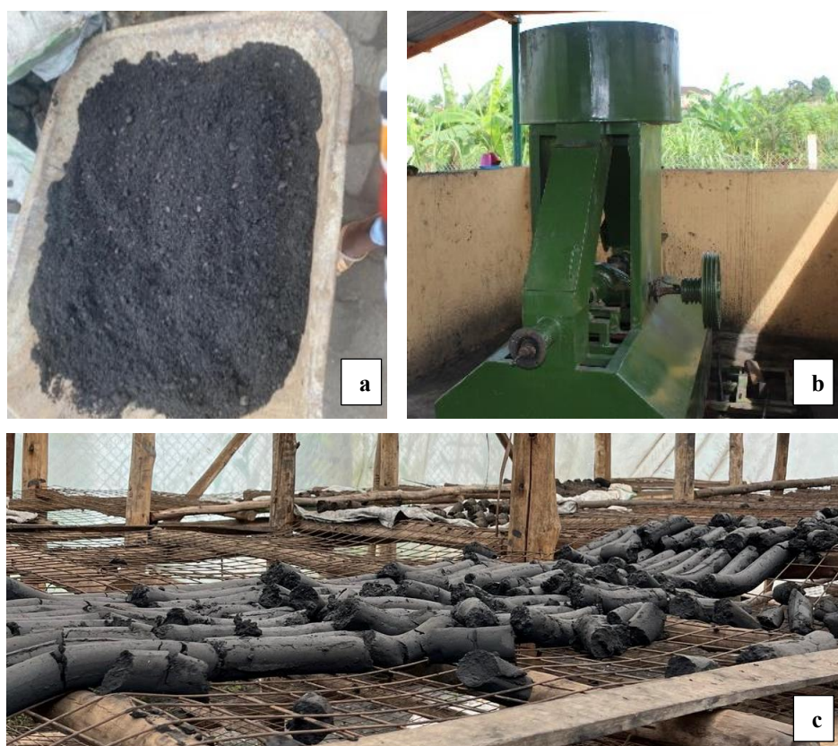
Figure 8.3: Photographs showing (a) ground char ready for extrusion; (b) the briquette extruder (Source: Water for People Uganda [used with permission]); and (c) produced briquettes on drying racks [photo taken April 2024].
