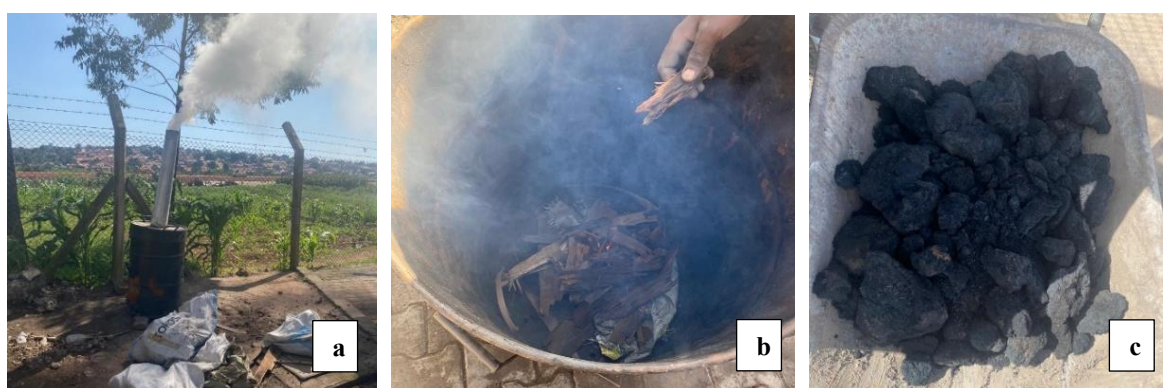
Figure 8.2: Photographs showing (a) the metallic drum kiln in use; (b) process initiation with wood as a start-up fuel; and (c) the produced faecal sludge char. Source: Water for People Uganda (used with permission).
