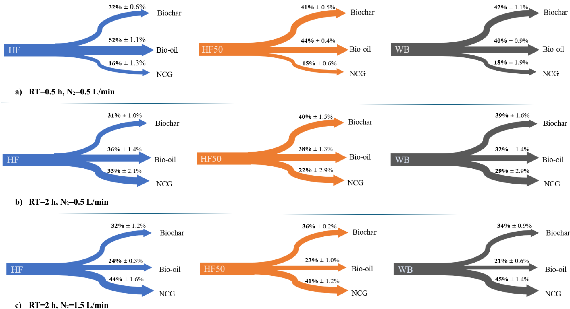
Figure 7.11: Distribution of carbon flows to biochar, bio-oil and non-condensable gas (NCG) streams expressed as the % of the total carbon content in the feedstock (for human faeces [HF], wood biomass [WB] and HF:WB 50:50 [HF50]) (pyrolysis at 550 °C). Results for different combinations of retention time (RT) at the highest heating temperature (550°C) and N 2 gas flow rate: (a) RT=0.5 h, N 2 =0.5 L/min; (b) RT=2 h, N 2 =0.5 L/min; and (c) RT=2 h, N 2 =1.5 L/min. The reported values are calculated based on Eq.7.1-7.3.
