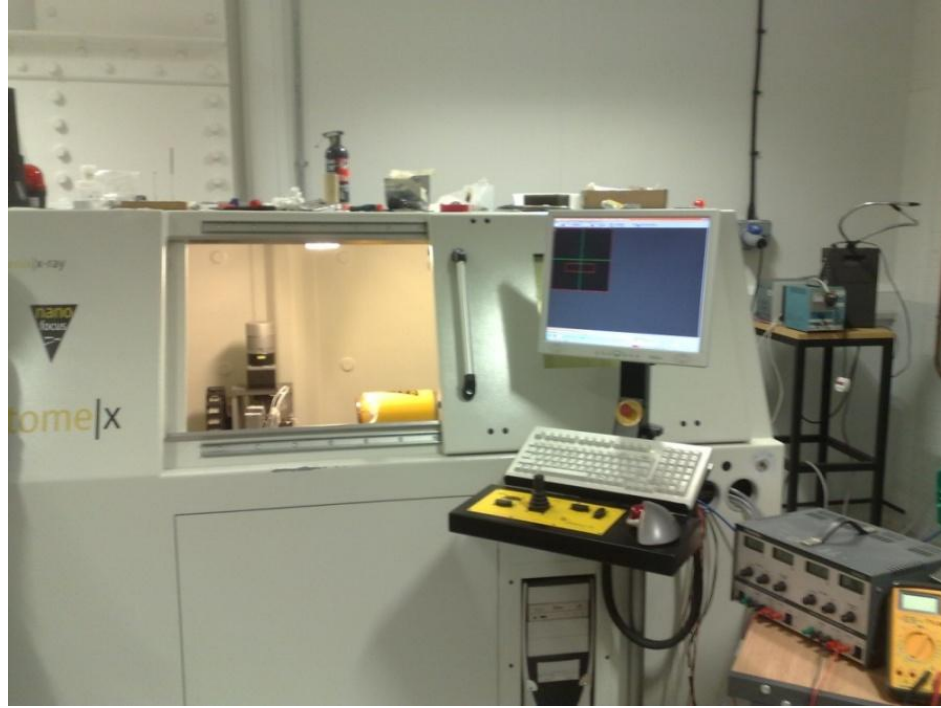
Figure 2.1: The micro-CT scanner at Imperial College that was used to capture the micro-structure of rock samples in this study.
