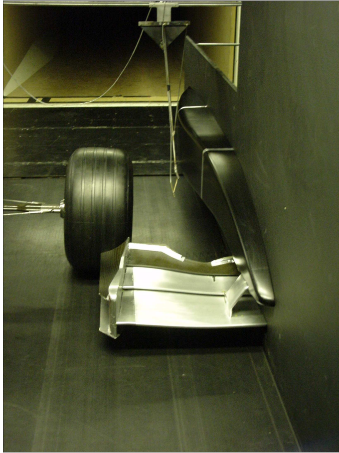
Figure 3.12: A photo of the McLaren model in the Donald Campbell tunnel showing the total pressure probe attached to the probe support and traverse
