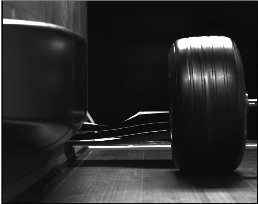
Figure 6.1: Field of view from flow visualisation camera located downstream of the model, highlighting the physical limitations on the visibility of flow in the near-field of the McLaren front wing and endplate
