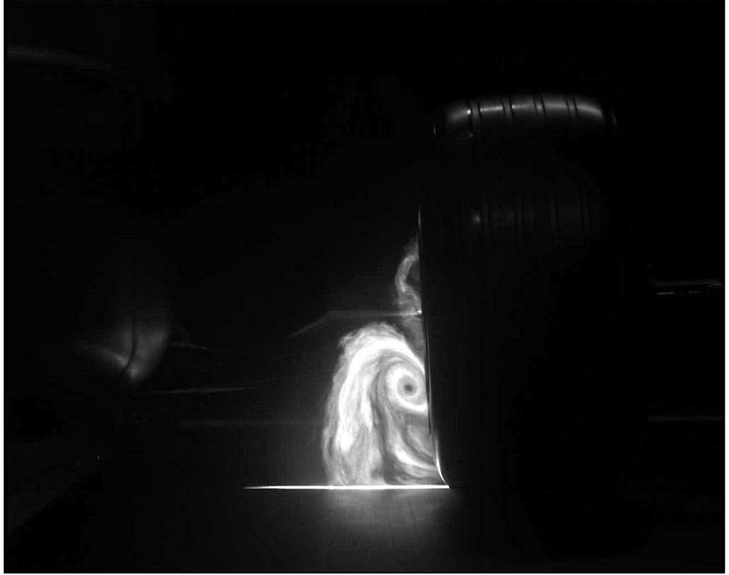
Figure 6.3: Laser smoke flow visualisation of flow in the near-field of the McLaren model ( Y = -250mmFS ) at a ride height of h/c_{mp} = 0.48 with rotating wheel ( V_{\infty} = 12.5m/s )
