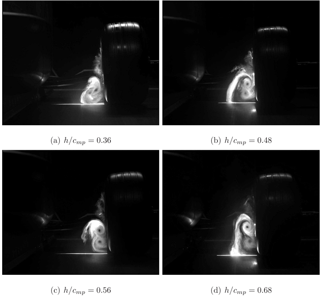
Figure 6.12: Laser-smoke flow visualisation at Y = -100mmFS downstream of McLaren model at varying ride height with the rotating wheel ( V_\infty = 12.5m/s )
