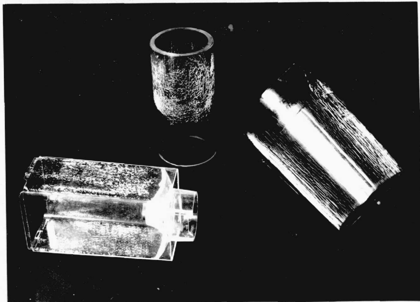
figure 3 1: Examples of Crazing in Practice
