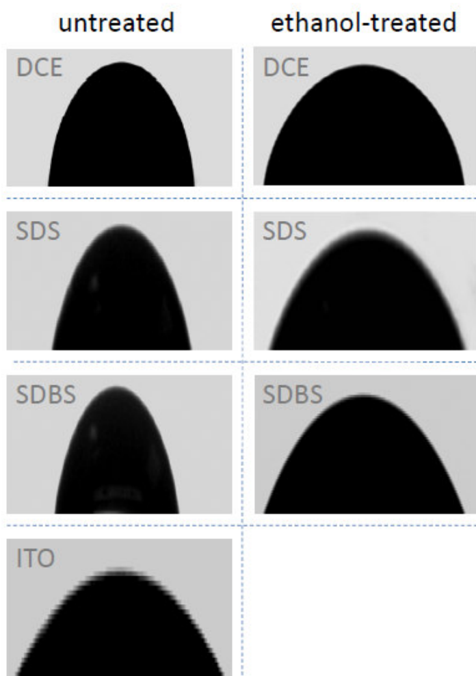
Figure 6.3 The wetting characteristics of the SWCNT films before (left) and after (right) spin-treatment with ethanol. In all cases there is a substantial reduction in contact angle after treatment, indicating improved wetting which is essential for subsequent deposition of PEDOT:PSS. The wetting characteristics for a water droplet on untreated ITO-coated glass are also shown for comparison.
