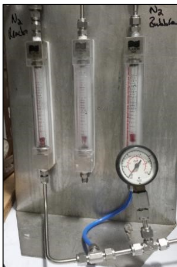
Fig. 4-5: Direct and indirect N 2 rotameters connected to the AFBR setup
