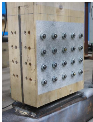
Figure 6.14 – Area of interest sprayed into a randomized pattern.
