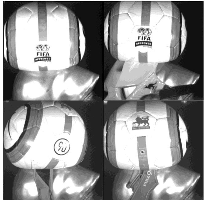
Figure 6: High Speed Video still of peak deflection.
