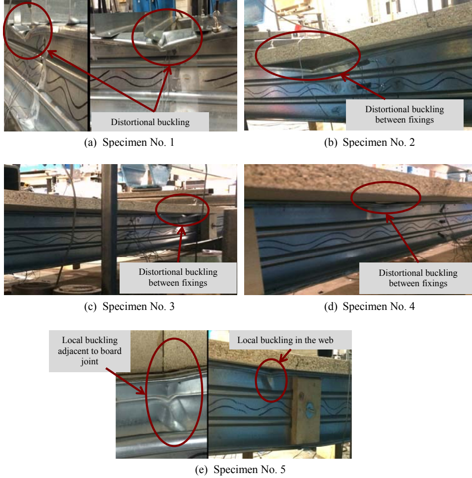
Fig. 11. Failure modes of 4-point bending specimens.
