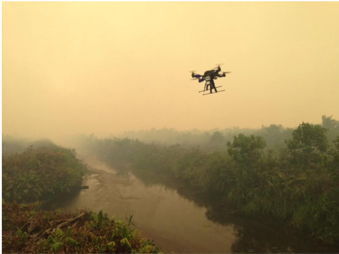
Figure 1: Remote-controlled drone over South Sumatra during the brief haze event of September-October 2014. Trace gas measurements from the drone are being used to better constrain emissions factors from tropical peat burning. (Courtesy Guido van der Werf, VU Amsterdam)
